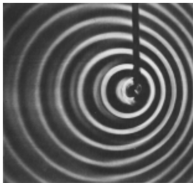
The pattern of waves made by a point source moving to the right across the water. Note the shorter wavelength of the forward-emitted waves and the longer wavelength of the backward-going ones.
