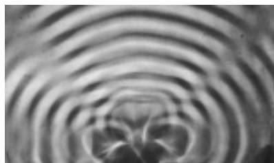
(c) A pretty good simulation of the single-slit pattern of figure (a), made by using three motors to produce overlapping ripples from three neighboring points in the water. (PSSC Physics)
