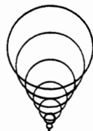
6.10 Coma as transverse ray aberration. The circles are loci of intersections of rays from a point object through concentric circles in the pupil. Once around a circle in the pupil corresponds to twice around the corresponding circle in the image.
