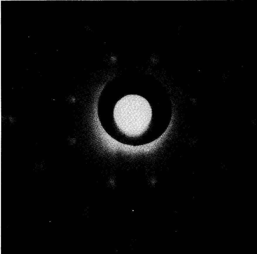
Fig. 9: Neutron Laue Pattern Taken with NaCl Crystal.
