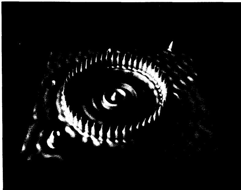
Figure 1.2 A “quantum corral” demonstrating the power of STM-type techniques (from Crommie et al. 1993). A ring of 48 Fe atoms, with a radius of about 140 \text{ \AA} , was constructed on the 111 surface of copper. The radial height variations were measured with the same technique and demonstrate the almost ideal nature of the surface on the inside of the ring. They result from the eigenstate of the corral.
