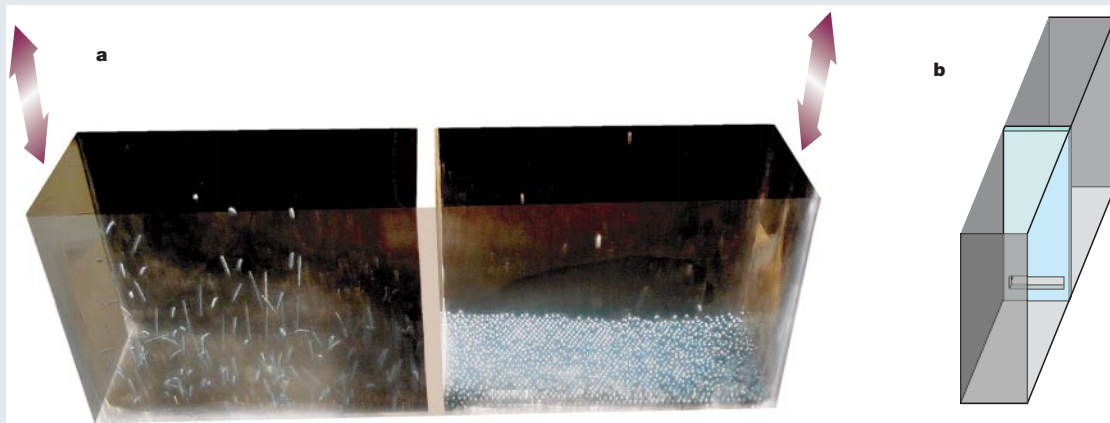
Figure 1 Separation of hot and cold beads in a granular 'Maxwell's Demon' experiment.
