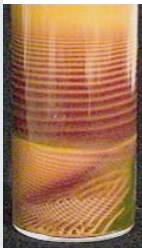
Box 1 Figure Liesegang patterns in a cylinder containing agar gel with dissolved K_2CrO_4 to which CuSO_4 has been added from above. See http://qsad.bu.edu/ogaf/lies/ for details of this system suitable for instructional use. (Photo: P. Garik, M. B. Gillespie and K. Brecher, Mathematics Education Center, Boston University.)
