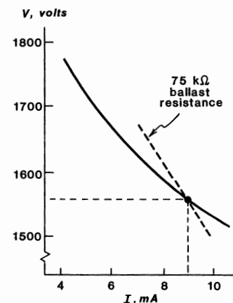
FIGURE 1.54 The glow discharge in a He-Ne laser tube has a negative-resistance I - V curve.
