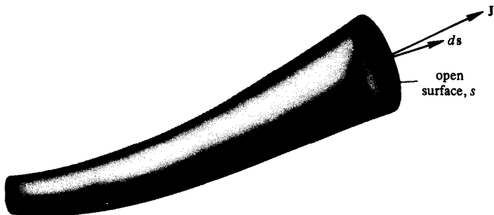
Figure 2.17. General current density \mathbf{J} over a cross section (open surface) s .
