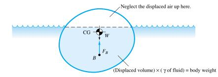
**Fig. 2.17** Static equilibrium of a floating body.
