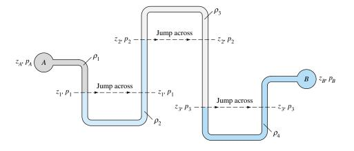
**Fig. 2.10** A complicated multiplefluid manometer to relate  $p_A$  to  $p_B$ . This system is not especially practical but makes a good homework or examination problem. difference in pressure between two chambers *A* and *B*. We repeatedly apply Eq. (2.20), jumping across at equal pressures when we come to a continuous mass of the same fluid. Thus, in Fig. 2.10, we compute four pressure differences while making three jumps:
