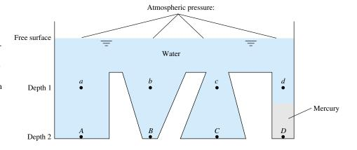
**Fig. 2.4** Hydrostatic-pressure distribution. Points a, b, c, and d are at equal depths in water and therefore have identical pressures. Points A, B, and C are also at equal depths in water and have identical pressures higher than a, b, c, and d. Point D has a different pressure from A, B, and C because it is not connected to them by a water path.
