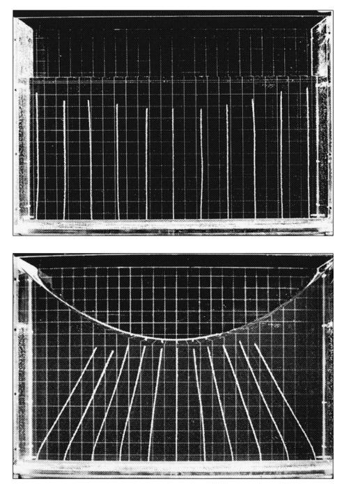
**Fig. 2.24** Experimental demonstration with buoyant streamers of the fluid force field in rigid-body rotation: (*top*) fluid at rest (streamers hang vertically upward); (*bottom*) rigid-body rotation (streamers are aligned with the direction of maximum pressure gradient). (*From Ref. 5, courtesy of R. Ian Fletcher.*)
