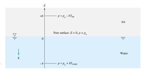
Fig. 2.5 Hydrostatic-pressure distribution in oceans and atmospheres.
