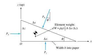
**Fig. 2.1** Equilibrium of a small wedge of fluid at rest.
