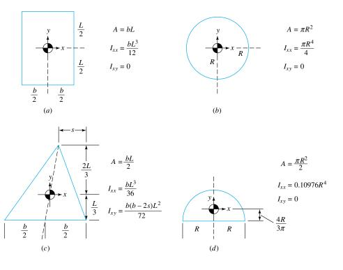
**Fig. 2.13** Centroidal moments of inertia for various cross sections: (*a*) rectangle, (*b*) circle, (*c*) triangle, and (*d*) semicircle.
