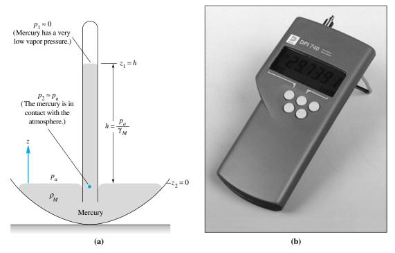
**Fig. 2.6** A barometer measures local absolute atmospheric pressure: (*a*) the height of a mercury column is proportional to  $p_{\text{atm}}$ ; (*b*) a modern portable barometer, with digital readout, uses the resonating silicon element of Fig. 2.28*c.* (*Courtesy of Paul Lupke, Druck Inc.*)
