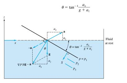
**Fig. 2.21** Tilting of constantpressure surfaces in a tank of liquid in rigid-body acceleration.
