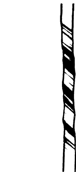
Fig. 30-12. A photograph of a small crystal of copper after stretching. [Courtesy of S. S. Brenner, Senior Scientist, United States Steel Research Center, Monroeville, Pa.]
