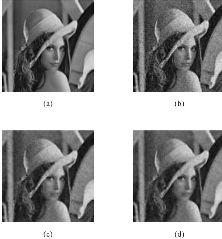
FIG. 6.4. Restoration of 256 grey-scale image by the Gaussian prior and edges (line process). Degradation was by Gaussian noise of vanishing mean and variance 900: (a) original image, (b) degraded images, (c) restored image by mean-field annealing, and (d) restored image by cluster variation method. Courtesy of Kazuyuki Tanaka (copyright 2001).
