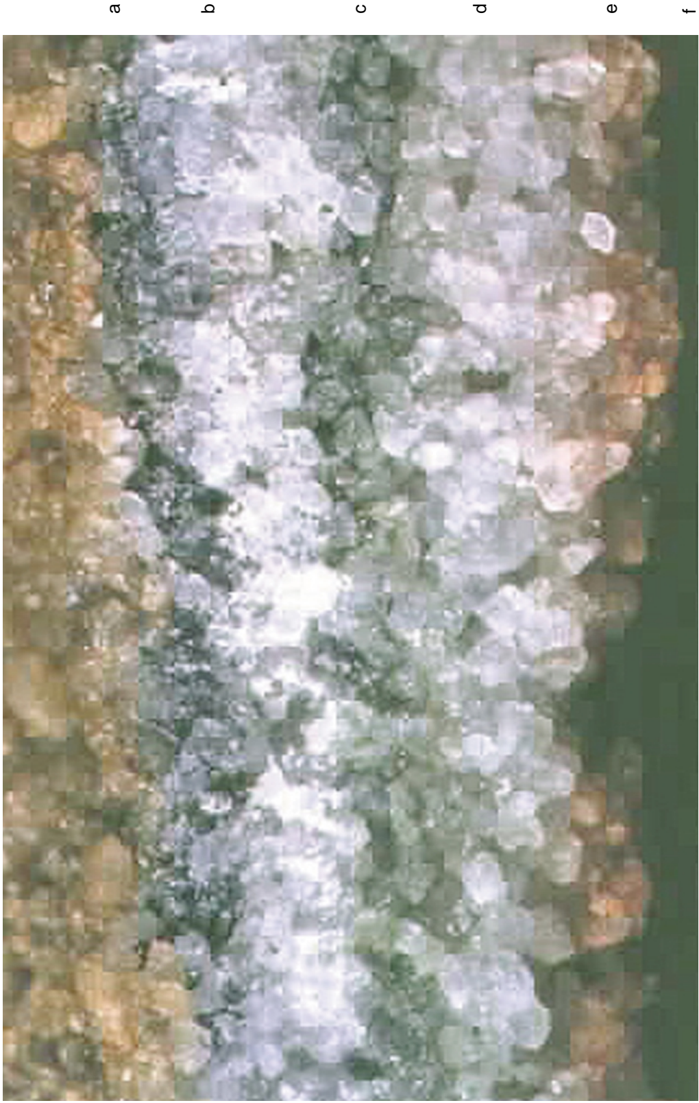
Plate 5.2 A cross-section (enlarged approximately 10 times) of a sandstone sample from East Beacon Ridge. Six distinct layers: a, b, c, d, e, and f are identified.
