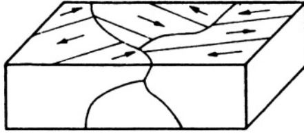
Figure 14.2.3. Domain structure in rolled polycrystalline Ni-Fe alloys. From Chikazumi et al. (1957).
