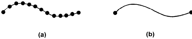
Figure 3.11. If we redistribute the mass in the mass–string system (a) along the string uniformly, we obtain homogeneous string in (b).
