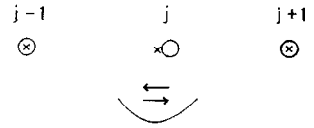
Figure 3.4. The j th atom in the linear chain executes simple harmonic oscillations as characterized by the Hamiltonian in Eq. (3.2.1).
