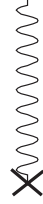
Fig. 1.5.4 - Graphical representation for an external electromagnetic field. The upper end of the line can be attached to any fermion line.
