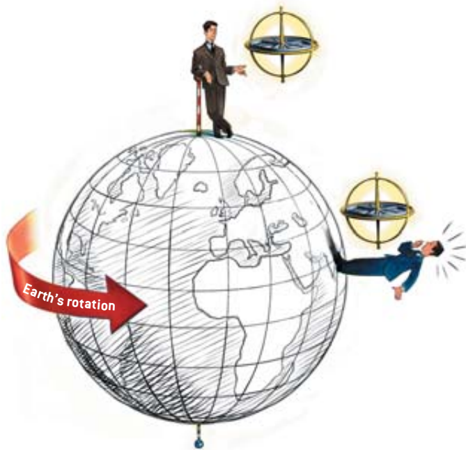
GYROSCOPIC DIRECTION FINDER , perfectly suspended so that it can rotate in any direction, will continue to point toward the same location in the heavens even as the earth spins and orbits. At any latitude away from the North Pole, however, as the earth turns, the gyro will leave the plane parallel to the ground—making it awkward to use for navigation.
