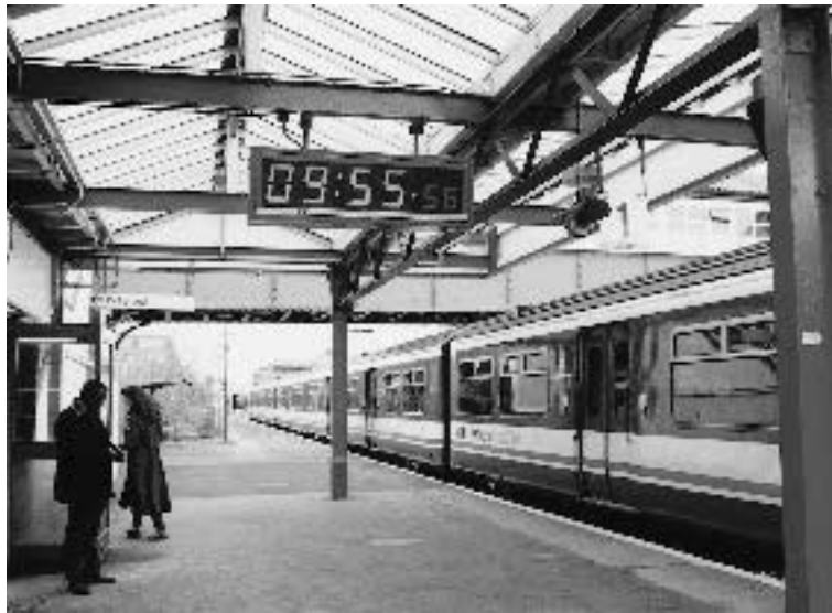
Figure 7.4. Railway clocks like this one are controlled directly by radio signals from the MSF transmitter.
