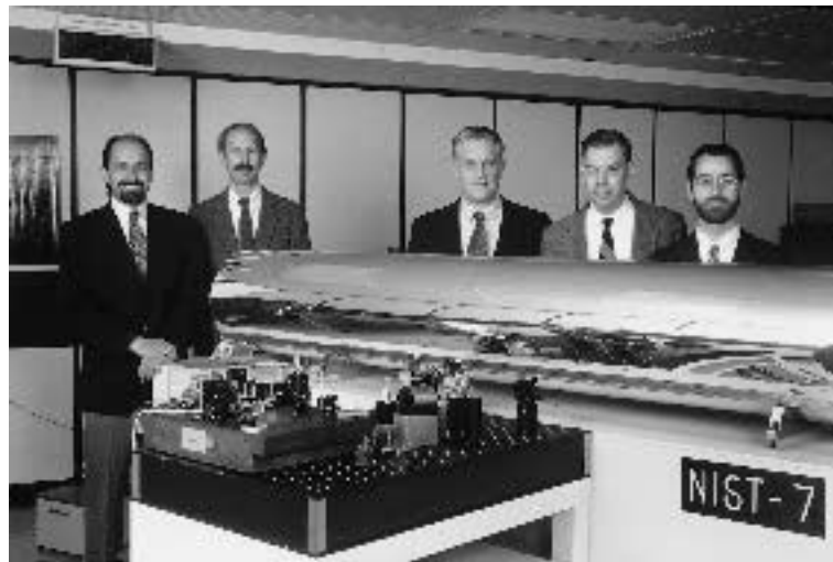
Figure 4.2. NIST-7, one of the most accurate atomic clocks in the world, is pictured here with its developers John P. Lowe, Robert E. Drullinger (project leader), David J. Glaze, Jon Shirley and David Lee of the US National Institute of Standards and Technology. It is an optically pumped caesium beam standard which is accurate to 2 seconds in 10 million years.
