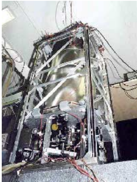
Figure 4.5. The first operational caesium fountain, LPTF-FO1, has been contributing to the world timekeeping system since 1995. Based at the Paris Observatory, the machine is currently the most accurate frequency standard in the world and can keep time to better than 1 second in 10 million years.
