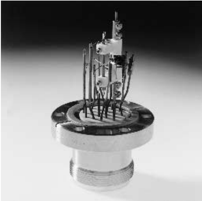
Figure 8.6. A trap constructed at NPL to confine ions of strontium or ytterbium. The ion is trapped between the two pointed electrodes above the centre of the picture.
