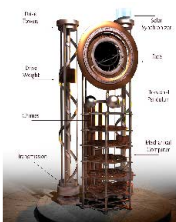
Figure 8.1. One of the proposed designs for the Clock of the Long Now, intended to run for 10 000 years. A small-scale prototype was finished in time to strike the third millennium.
