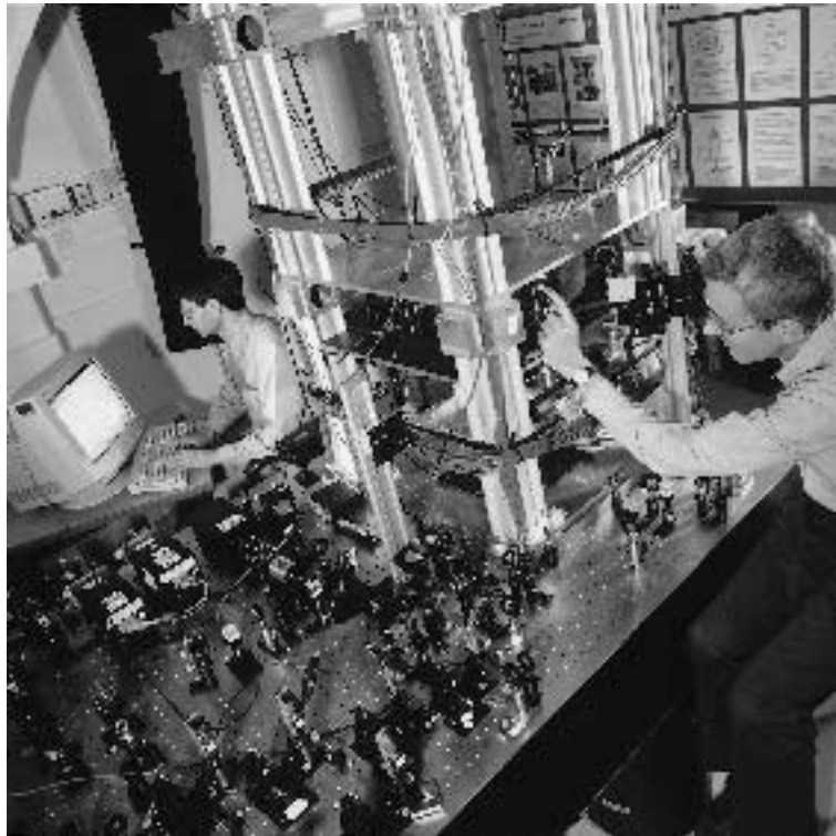
Figure 8.2. Peter Whibberley (left) and Dale Henderson at work on the experimental caesium fountain at NPL. The fountain itself is contained within the rectangular framework above centre, while the optics to the bottom left are used to prepare the laser beams. The laboratory was once used for calibrating marine chronometers.
