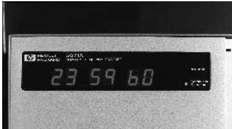
Figure 5.7. The last minute of 1998 had 61 seconds. The leap second was caught by this atomic clock at NPL.
