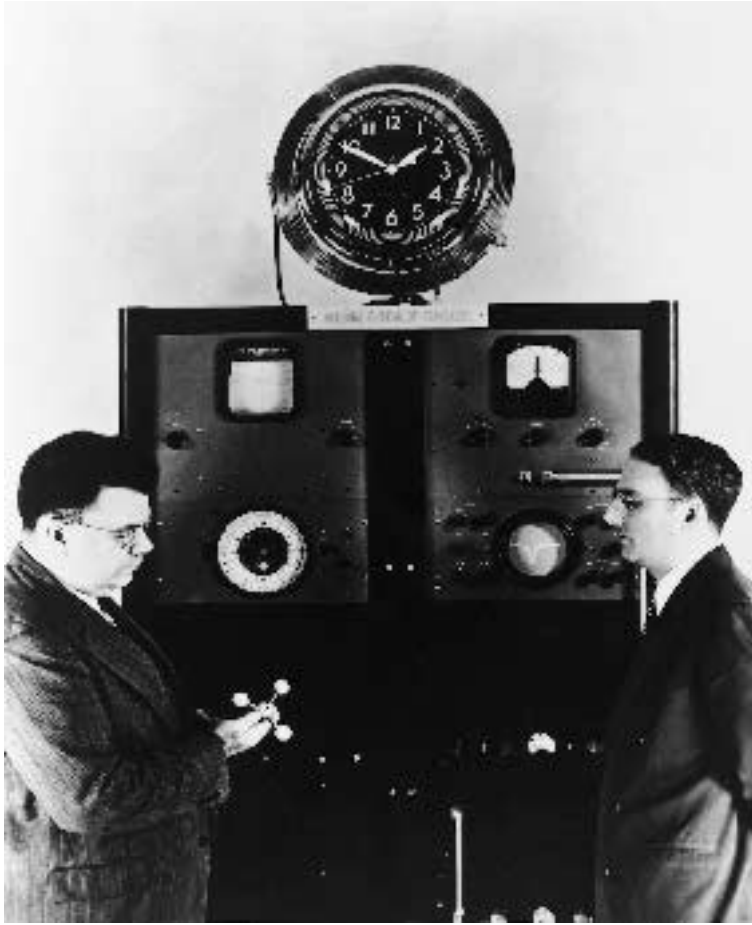
Figure 2.10. The world's first atomic clock is unveiled at the US National Bureau of Standards in 1949. It was based on the absorption of radio waves by ammonia gas at a frequency of 23 870 megahertz. NBS director Edward Condon (left) examines a model of the ammonia molecule while the clock's designer, Harold Lyons, looks on.
