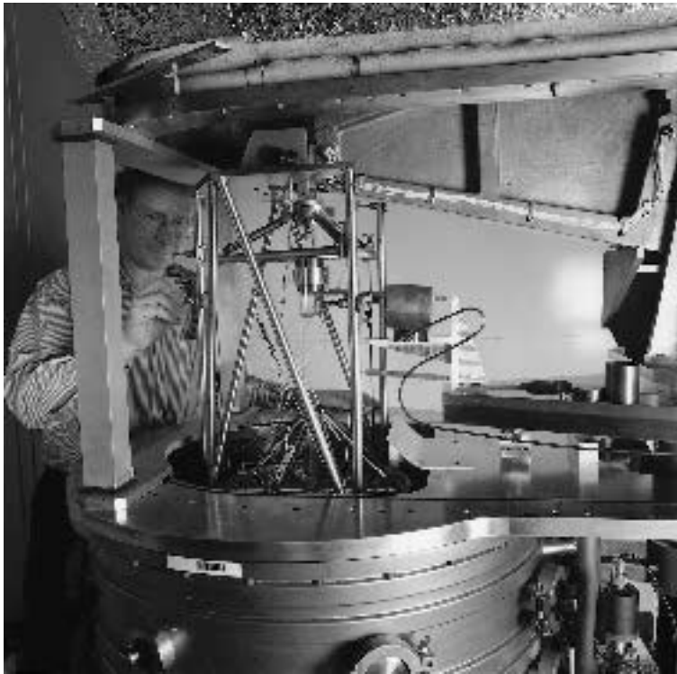
Figure 7.7. This apparatus, known as a Watt balance, is being used at NPL in a series of experiments that may ultimately lead to the kilogram being redefined in terms of the caesium frequency.
