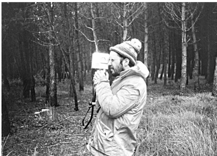
Figure 9.6 EM-16 in normal reading position.
