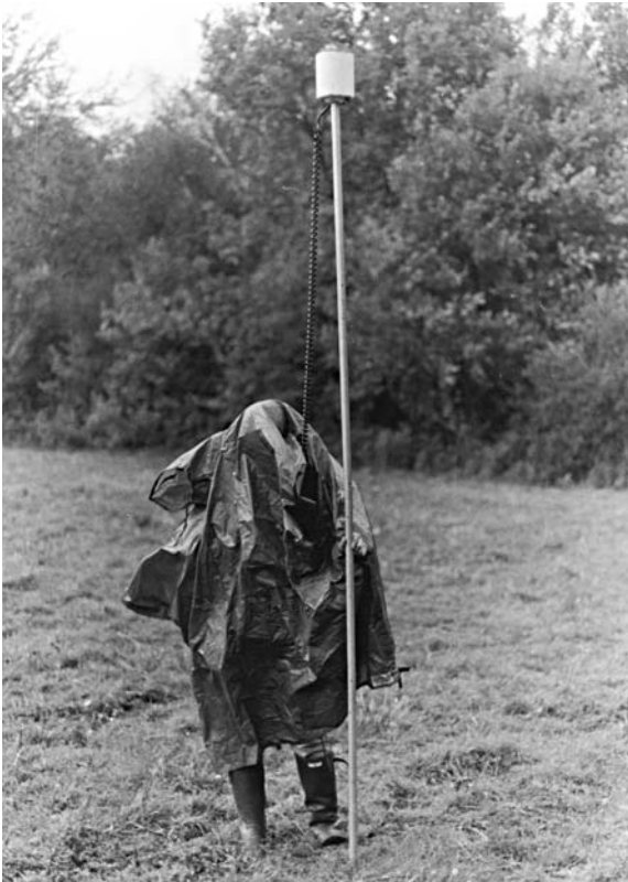
Figure 1.6 The geophysical cape in action. Magnetometer and observer are both dry, with only the sensor bottle exposed to the elements.
