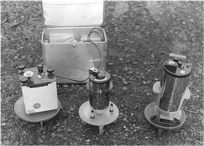
Figure 2.3 ‘Manual’ gravity meters. From left to right, LaCoste ‘G’ (geodetic), Worden ‘Student’ and Sodin.
