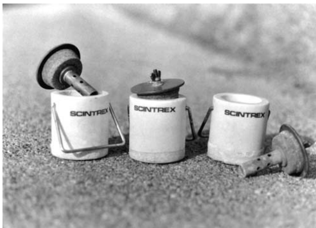
Figure 5.4 Porous-pot non-polarizing electrodes designed to be pushed into a shallow scraping made by a boot heel. Other types can be pushed into a hole made by a crowbar or geological pick.
