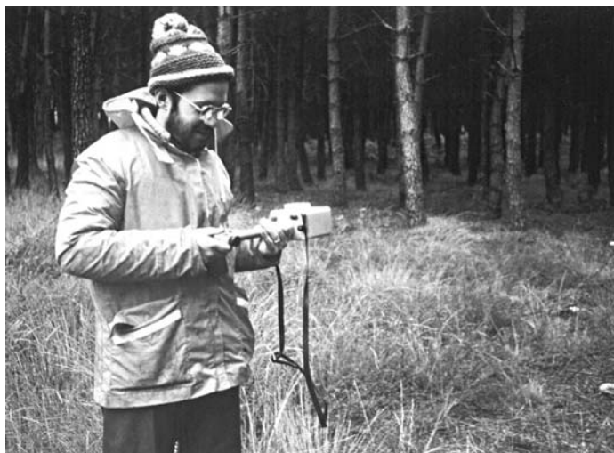
Figure 9.7 Searching for the station with the EM-16.
