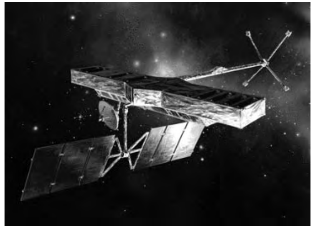
Figure 2. Artist's impression of the Space Interferometry Mission in orbit. The main structure houses the optical telescopes and Michelson interferometric beam combiner. The boom supports a system of laser metrology gauges which monitor the exact positions of the first optical elements in each telescope, a 40 cm siderostat. (Figure courtesy of Jet Propulsion Laboratory, California Institute of Technology.)
