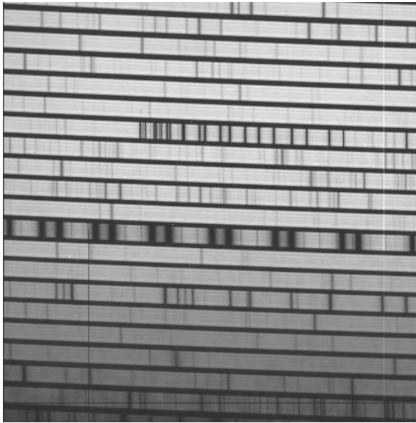
Figure 2. A typical echelle spectrogram: sunlight at the 2dcoudé spectrograph of the McDonald Observatory 2.7 m telescope. The resolving power is R = \lambda/d\lambda = 200\,000 . The spectrum was exposed on a 2048 \times 2048 Tektronic, Inc, CCD. The image covers a fraction of the observable spectrum in echelle spectral orders 56–36 (top to bottom) covering parts of the wavelength region 6126 \text{ \AA} - 9550 \text{ \AA} in the red and near infrared. The strong, broad lines in order 45 (near the centre of the figure) and the strong sharper lines in order 50 are the 'A' and 'B' bands of molecular oxygen in the Earth's atmosphere. Atmospheric water vapor produced the strong lines in order 42.
