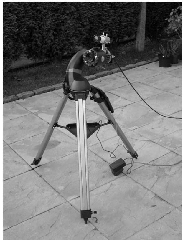
Figure 3. 135mm focal length lens and Starlight Express MX-516 CCD on a Celestron NexStar GoTo tripod mounting.
