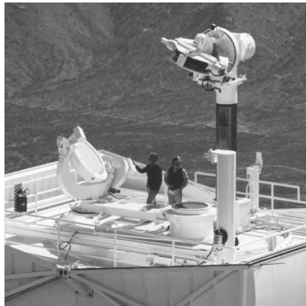
Figure 1. Large coelostat feed for the Kitt Peak Vacuum Telescope. Here the number 2 mirror is adjustable in height and angle only. The coelostat itself swings along a circular path to account for seasonal and diurnal change. This scheme was first used at the Potsdam Observatory in Germany.
