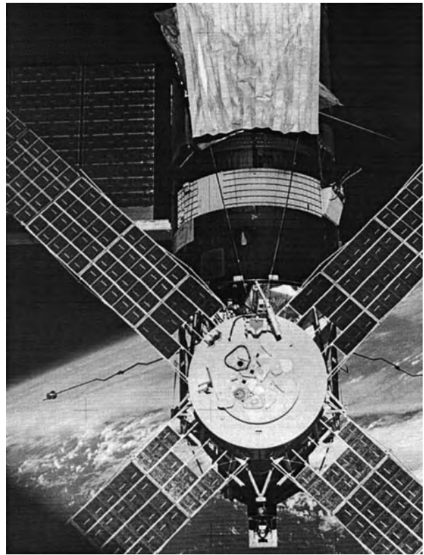
Figure 1. View of Skylab from the Sun. The OWS is at the top, covered with a parasol and sunshade. The one OWS solar array is at the upper left; the diagonal arrays supplied power to ATM. The ATM doors and experiment access ports are shown in the circular structure at the lower center. From Eddy (1979).
