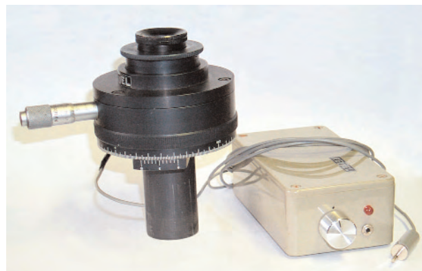
Figure 3. The RETEL filar micrometer used by the writer. It uses parallel wires (one movable and one fixed) to measure separation and a third wire at right angles to measure position angle. The whole field is illuminated by means of a variable-intensity red light-emitting diode. Credit: Richard Sword, Institute of Astronomy, Cambridge.
