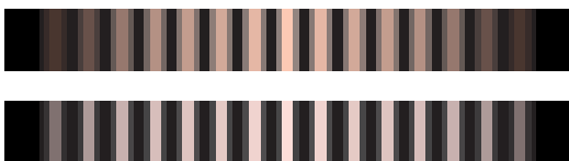
(d) A double-slit diffraction pattern (top), and a triple-slit pattern (bottom).
