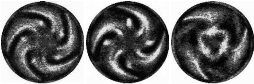
Fig. 11. Flow visualisation of the wide gap flow structures for \beta = 0.5 (view on the polar region): spiral wave flow with m = 5 ( Re = 1320 ), m = 4 ( Re = 1575 ) and m = 3 ( Re = 1680 )
