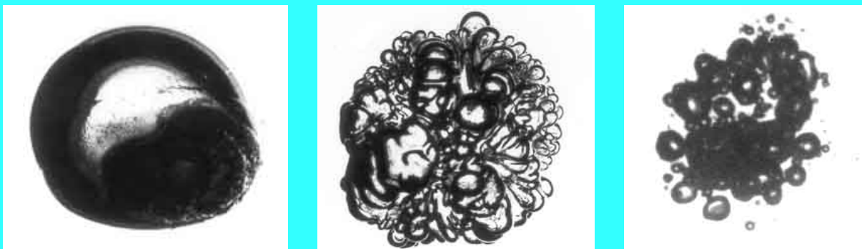
Figure 3.3 Photographs of an ether bubble in glycerine before (left) and after (center) a collapse and rebound. The cloud on the right is the result of a succession of collapse and rebound cycles. Reproduced from Frost and Sturtevant (1986) with the permission of the authors.
