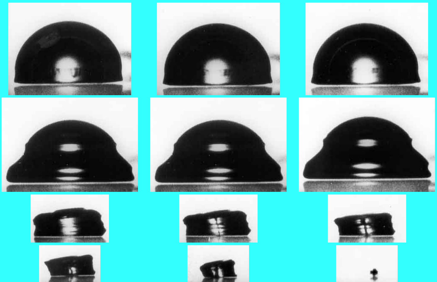
Figure 3.10 Series of photographs of a hemispherical bubble collapsing against a wall showing the "pancaking" mode of collapse. Four groups of three closely spaced photographs beginning at top left and ending at the bottom right. From Benjamin and Ellis (1966) reproduced with permission of the first author.
