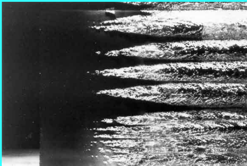
Figure 7.19 Streak cavitation on a biconvex hydrofoil at a speed of 15.5m/s and a cavitation number of 0.11 (Arakeri 1975). The flow is from left to right and the leading edge of the foil is about 1cm from the left-hand edge. Reproduced with the permission of V.H. Arakeri.
