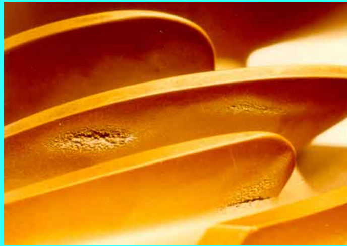
Figure 3.11 Photograph of typical cavitation damage on the blade of a mixed flow pump.
