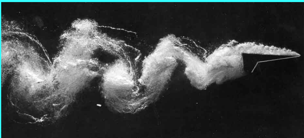
Figure 7.11 Cavitating vortices in the separated wake of a lifting flat plate with a flap; the flow is from the right to the left. Reproduced with the permission of A.J. Acosta.
