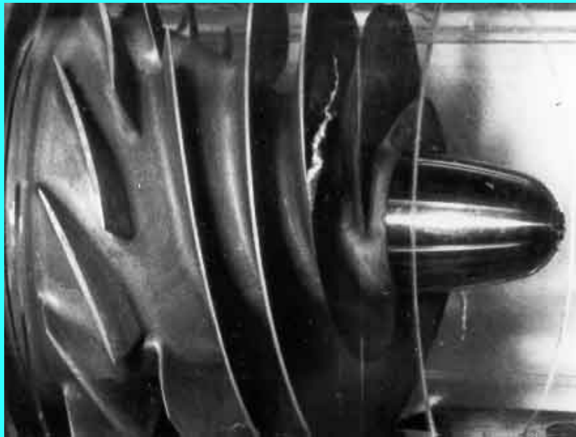
Figure 7.8 Cavitating tip vortex on a scale model of the low-pressure LOX turbopump impeller in the Space Shuttle Main Engine. The fluid is water, the inlet flow coefficient is 0.07 and the cavitation number is 0.42. Reproduced from Braisted (1979).
