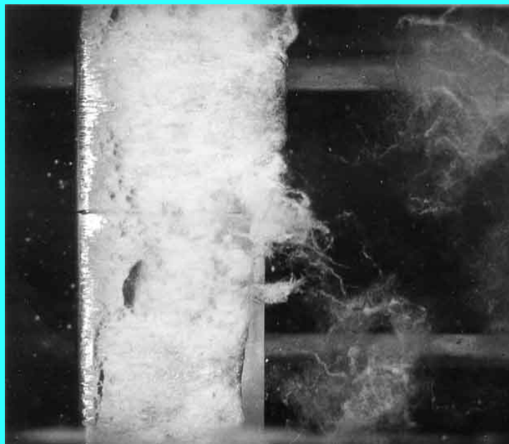
Figure 7.15 Sheet cavitation on the suction surface of a NACA 4412 hydrofoil at an angle of attack of 12^\circ , a speed of 10.7m/s and a cavitation number of 1.05 (Kermeen 1956). The flow is from left to right.
