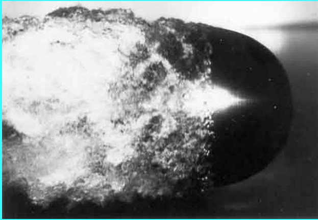
Figure 7.16 Two photographs of a cavitating, 7.62cm diameter sphere. The left photograph shows bubble cavitation and bubbly wake prior to the transition to the fully developed cavity shown on the right (Brennen 1970). The flow is from right to left, the velocities being 5.6m/s and 10.7m/s, respectively.
