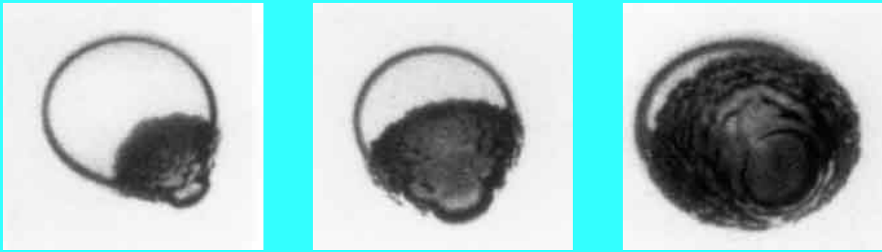
Figure 2.10 Typical photographs of a rapidly growing bubble in a droplet of superheated ether suspended in glycerine. The bubble is the dark, rough mass; the droplet is clear and transparent. The photographs, which are of different events, were taken 31, 44, and 58 \mu s after nucleation and the droplets are approximately 2mm in diameter. Reproduced from Frost and Sturtevant (1986) with the permission of the authors.
