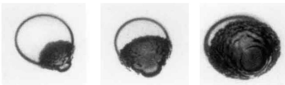
Figure 2.10: Typical photographs of a rapidly growing bubble in a droplet of superheated ether suspended in glycerine. The bubble is the dark, rough mass; the droplet is clear and transparent. The photographs, which are of different events, were taken 31, 44, and 58 \mu s after nucleation and the droplets are approximately 2mm in diameter. Reproduced from Frost and Sturtevant (1986) with the permission of the authors.
