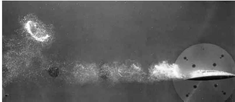
Figure 7.13: A vortex ring shed by the partial cavitation oscillations of a hydrofoil. The flow is from right to left. Reproduced with the permission of A.J. Acosta.
