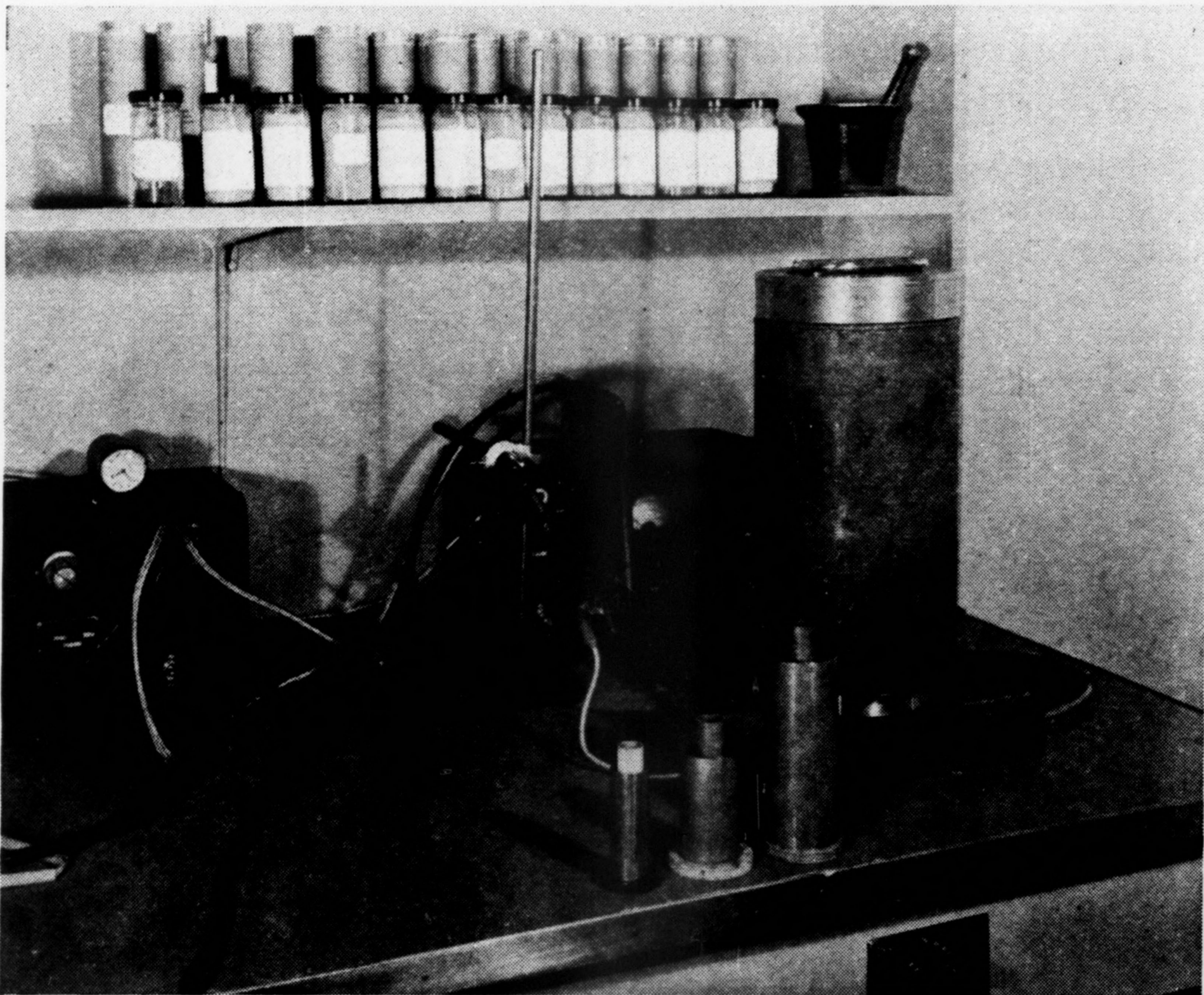
FIG. 2. Containers 1, 2, 3, and Geiger Counter shielded by lead.
