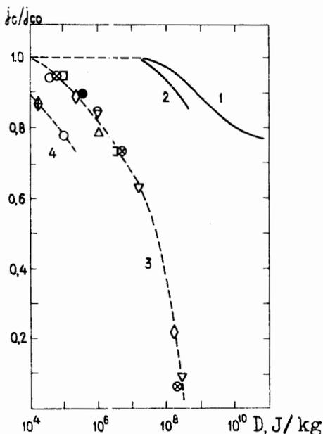
Fig. 1. Dependence  $j_c(D)/j_{c0}(D)$  for the low temperature NbTi superconductors irradiated by reactor neutrons (1) and protons with energy 30 GeV (2), and for the HTSC-ceramics  $YBa_2Cu_3O_7$  irradiated by protons with energy 0.66 and 8.09 GeV (3) or nuclei  $^{12}C$  with energy 3.65 GeV/nucleon (4). Denotations are indicated in the table.
