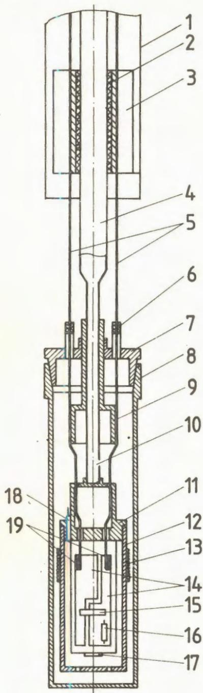
Fig. 1. The lower part of the set-up. 1 - external stainless tube, 2 - insulating gasket 3 - heat drain for terminals and current leads, 4 - constructive stainless tube, 5 - current leads, 6 - leak-tight inlets of current leads, 7, 8 - chamber, 9 - heat drain, 10 - pumping tube, 11 - sample holder, 12 - heat screen, 13 - heater, 14 - current electrodes, 15 - sample, 16 - TVO thermometer, 17 - Hall's sensor, 18 - capacitive thermometer, 19 - current lead soldering.
