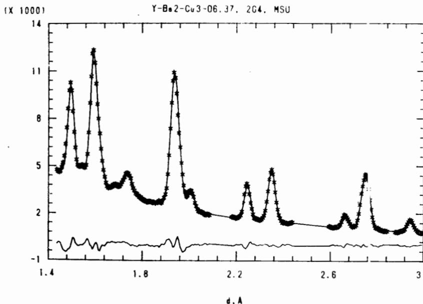
Fig. 1. Observed (dots) and calculated (solid line) diffraction profile from sample No. 3. The difference curve is shown in the bottom. The total of 245 experimental points were processed with R-factor over profile being 2.6%, weighted  $R_w$ -factor 3.4% and expected  $R_e = 2.1\%$ .
