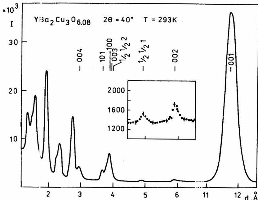
Fig.2. Diffraction spectrum from sample No.4 measured at  $2\theta=40^\circ$ . A peak at  $d=4.93 \text{ \AA}$  is clearly observable. It may be considered as  $(1/2 \ 1/2 \ 1)$  magnetic reflection from the AF structure.
