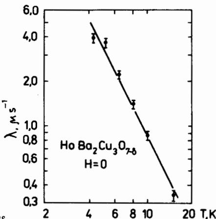
Fig.3. Temperature dependence of  $\lambda(T)$  in the temperature range 4.2-15 K. The solid line is plotted according to formula (2).
