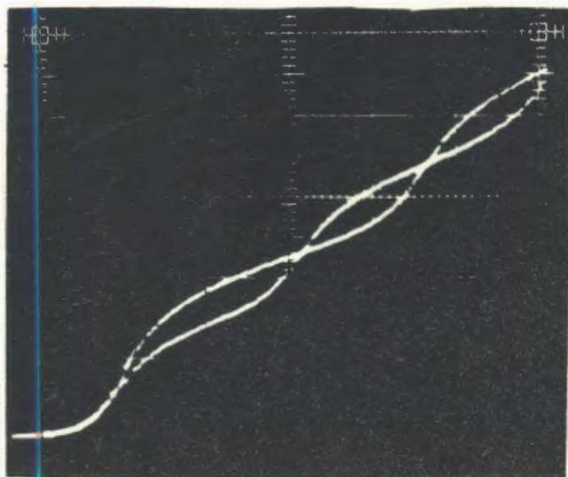
Fig. 2. Voltage-current characteristic of ceramic 2-hole rf-squid, operating at 78 K. X-axis - squid pumping amplitude. Y-axis - squid signal amplitude.
