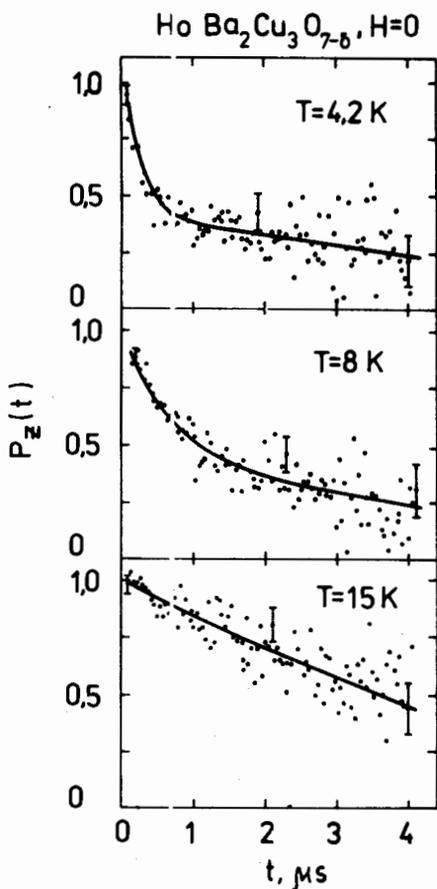
Fig.1. Muon spin relaxation functions in  $\text{HoBa}_2\text{Cu}_3\text{O}_{7-\delta}$  at different temperatures in the zero external magnetic field. The solid curves are plotted according to formula (1).
