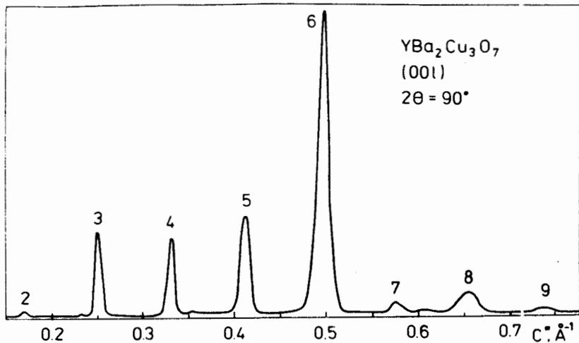
Fig. 2. The orders of the reflection from (001) plane of the  $YBa_2Cu_3O_7$  single crystal.
