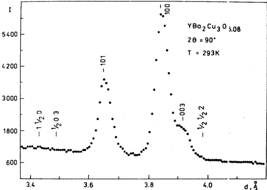
Fig.3. Diffraction spectrum from sample No.4. In the vicinity of  $d=3.99 \text{ \AA}$  the  $(1/2 \ 1/2 \ 2)$  magnetic reflection must occur, but its intensity does not exceed the statistical error.
