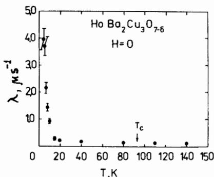
Fig.2. Temperature dependence of the muon spin relaxation rate  $\lambda$  in the zero external magnetic field.
