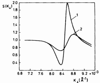
of oxygen near a film surface may cause the existence of such a layer. Figure 3 demonstrates the manner in which  $S(k_{\perp})$  depending on  $\delta$  is changing.
