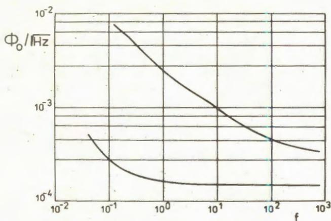
Fig. 4. Fourier-spectrum of ceramic 2-hole rf-squid at 78 K (upper curve) and of standard low-temperature 2-hole rf-squid at 4 K (lower curve). X-axis - frequency, Hz. Y-axis - noise density,  $\Phi_0/\text{Hz}^{1/2}$ .
