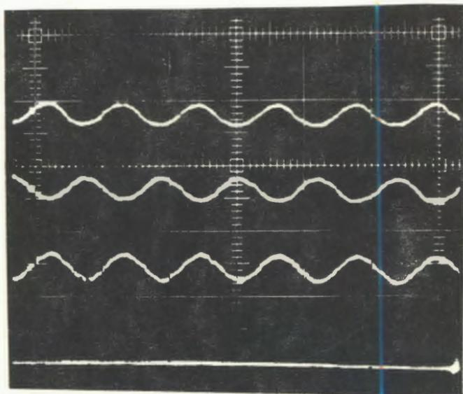
Fig. 3. A 2-hole rf-squid signal dependence on applied external magnetic field, received in the first 3 plateaus. Operating temperature - 78 K. Bandwidth - 1KHz. X-axis - magnetic field, 3.1 nT/div. Y-axis - squid signal, 20  $\mu$ V/div.
