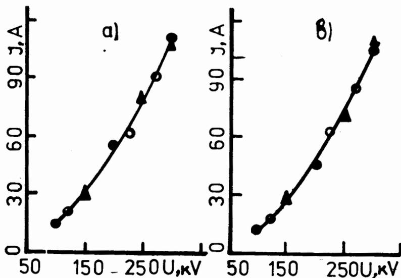
Fig. 1. Voltage-current characteristics of electron source diode with cathode made of  $Y_1Ba_2Cu_3O_{7-\delta}$  for  $t_1 \sim 300$  K (a) and  $t_2 \sim 79$  K (b) and for:  $\circ - \rho \sim 2.5 \times 10^{-2} \Omega \cdot \text{cm}$ ;  $\bullet - \rho \sim 10^{-1} \Omega \cdot \text{cm}$ ;  $\blacktriangle - \rho \sim 2 \Omega \cdot \text{cm}$ .
