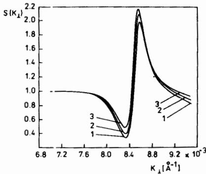
Fig.4.  $S(k_{\perp})$  for an ideal reflectometer (curve 1) and considering finite resolution (curve 2). A film with a thickness of  $1000 \text{ \AA}$ , in a field  $H=420$  gauss and  $\Lambda=200 \text{ \AA}$ .
