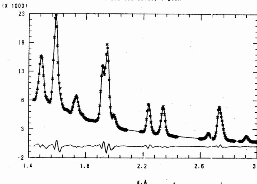
Fig. 1. The observed (stars) and calculated (solid line) neutron profile intensities for  $\text{YBa}_2\text{Cu}_3\text{O}_{7-\delta}$  with the difference marked below. The total number of points are 245,  $R = 2.7\%$ , the expected agreement index  $R_e = 1.8\%$ .
