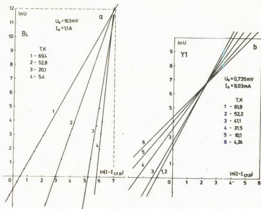
Fig. 4. The low voltage ( $U < 1 \text{ mV}$ ) parts of the IVC: a) Bi, b) Y1.
