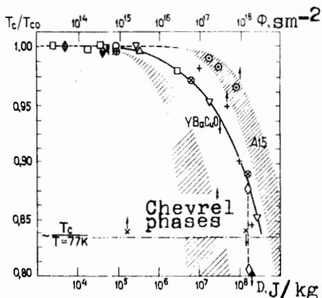
Fig. 2. Dependence  $T_c(D)/T_{c0}(D)$  for the HTSC-ceramics  $YBa_2Cu_3O_7$  under irradiation: a) by protons and  $^{12}C$  nuclei (solid curve with experimental points on it, symbols being explained in the table); b) by neutrons with  $E_n > 0.1$  MeV (the data on single-phase ceramics (+) and monocrystal (O) are given); c) by  $\alpha$ -particles with  $E_\alpha = 6.1$  MeV (the results are obtained with a film 1-2  $\mu m$  thick ( $\nabla$ )).
