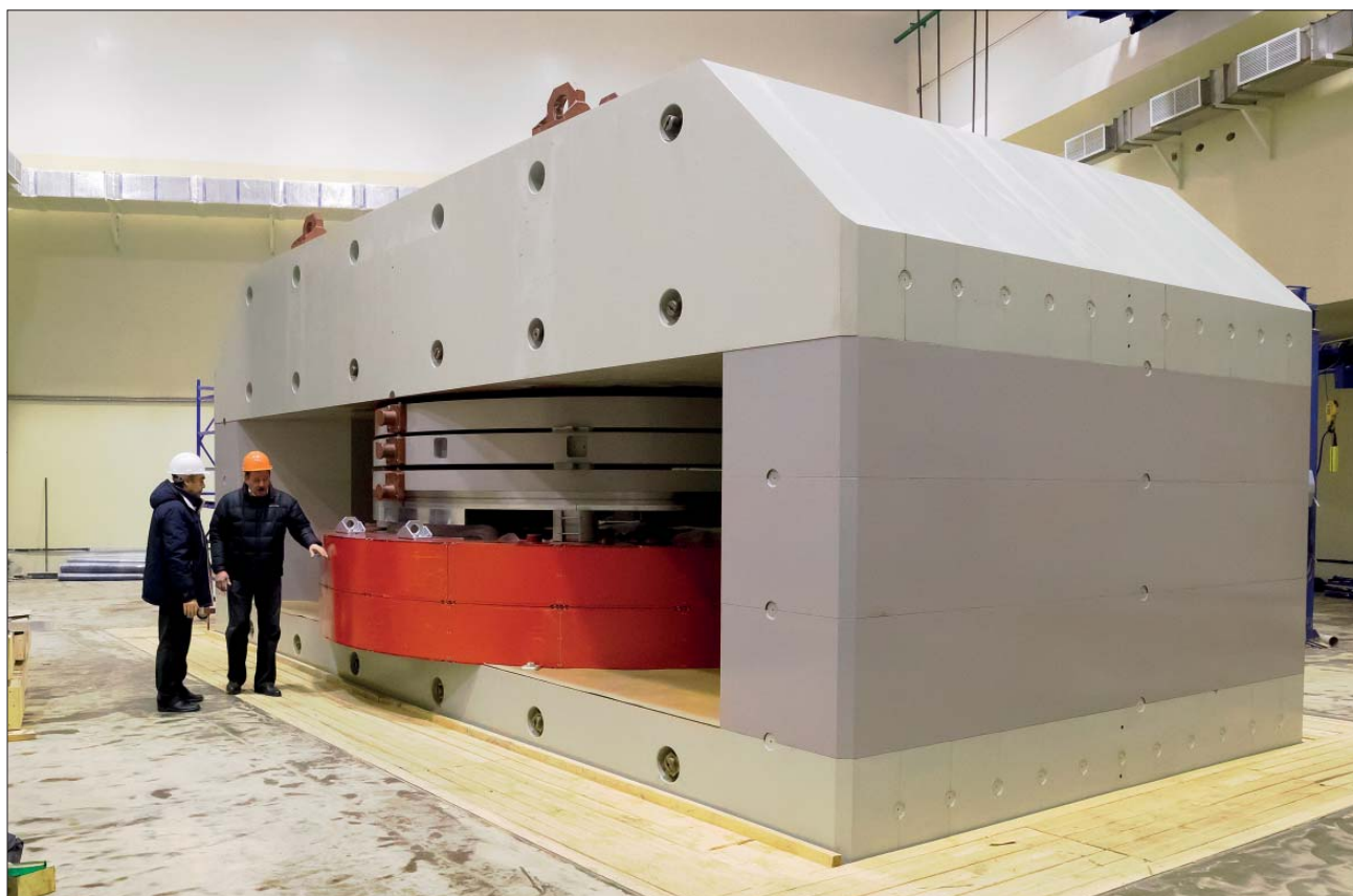
The Flerov Laboratory of Nuclear Reactions, 15 September. The assembling of the DC-280 cyclotron magnet in the building of the SHE factory
