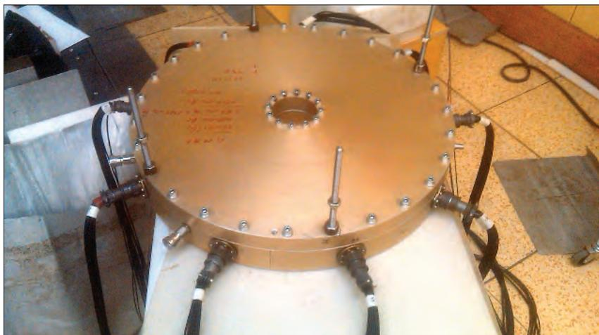
Fig. 2. The ring-shaped multi-section detector on a test bench
