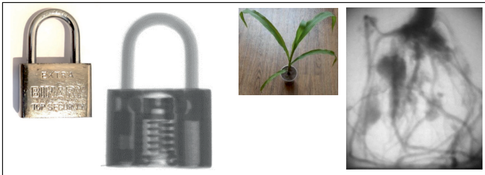
Fig. 2. Left: photo and neutron imaging of the metal padlock. Right: photo of the corn and the neutron radiographic image of the roots of the corn plant in the plastic container
