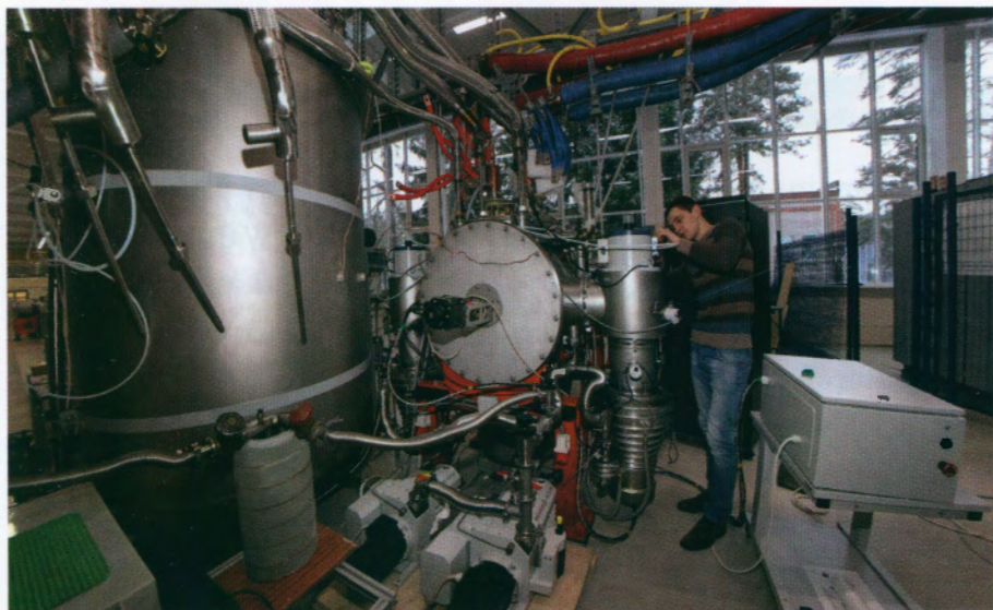
The booster dipole magnet test in the frames of the NICA project
