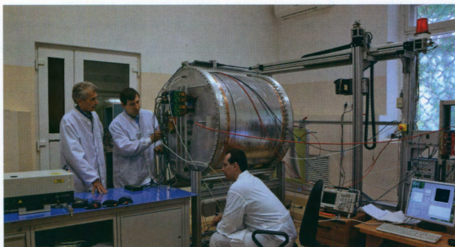
The Prototype of the time projection chamber TPC for the MPD NICA
