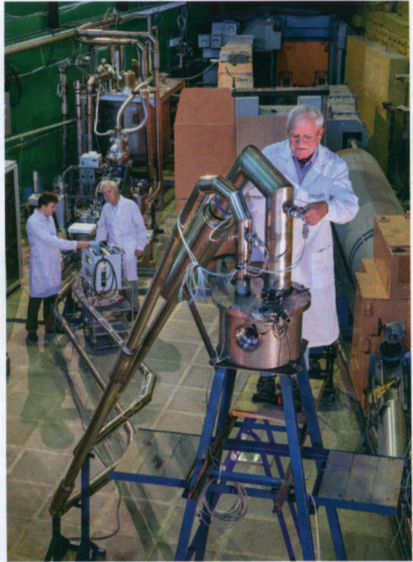
A test bench of the cryogenic neutron moderator of IBR-2
