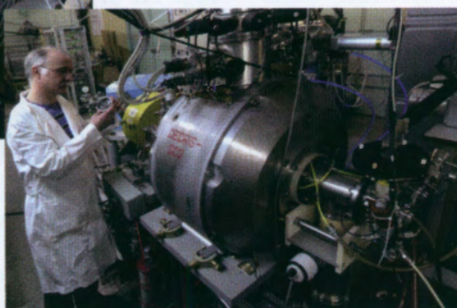
Superconducting magnetic system for the ECR source
