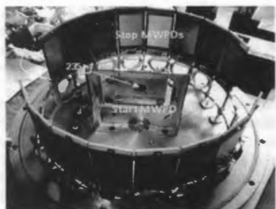
Fig.2. The experimental setup: left – the photo of reaction chamber with MWPD detectors; right - schematic view of the experiment.
