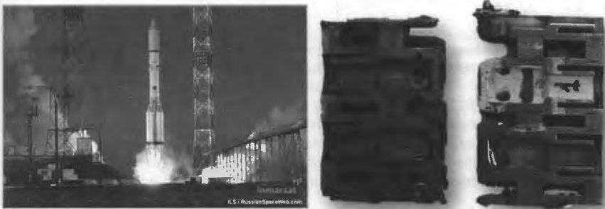
Fig. 3. The Proton-M rocket (left) and the photo of the part of the rocket engine (right). The piece containing palladium is marked as "1".
