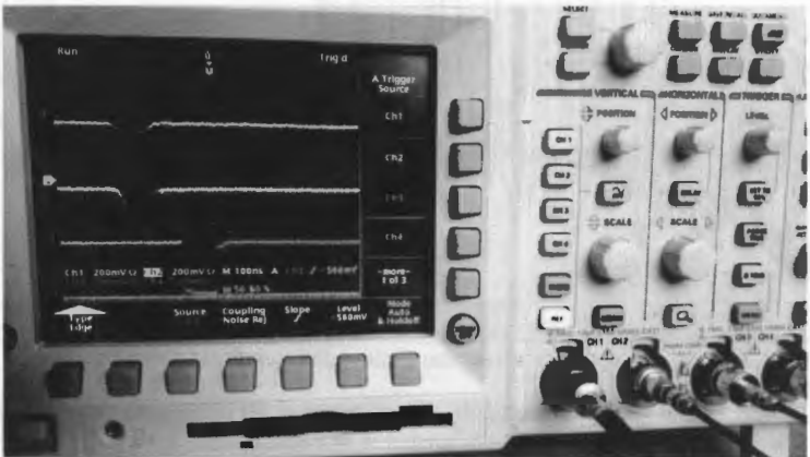
Fig. 14: testing of scintillator signals using Co-60 gamma ray source.
