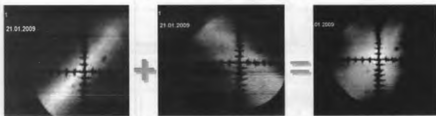
Fig.8. Beam spot on luminescent screen in front of the target: quadruple lenses doublet effect.
