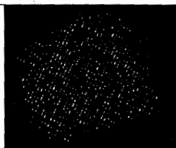
Fig.4 Ab initio reconstruction of overall \text{CoFe}_2\text{O}_4 nanoparticles shape for the ferrofluid sample of 0.5 % particle vol. concentration.
