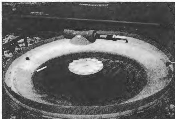
Figure 3. Special containers housed fish eggs and were exposed under known geometries with doses measured by TLDs. The photo depicts one of several egg exposure arrangements that were tested.
