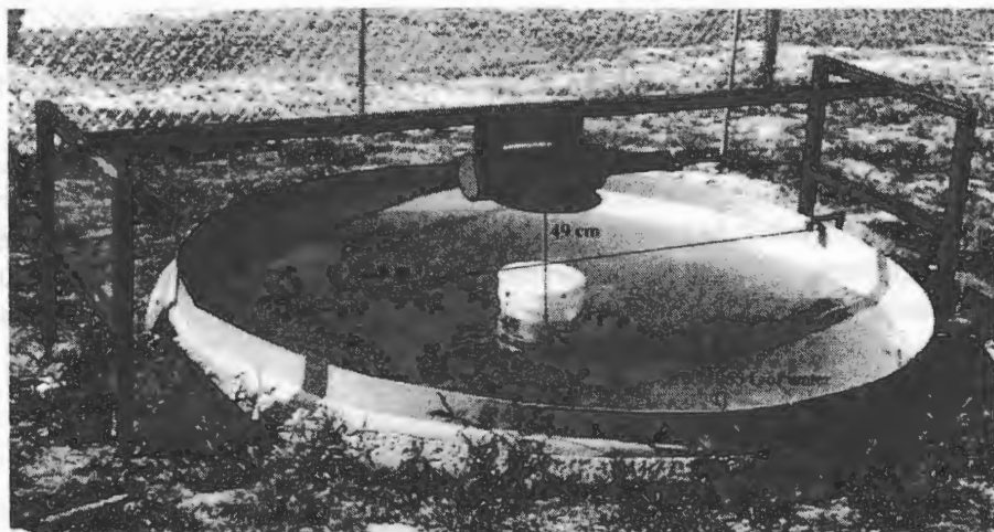
Figure 1. Photo of a single mesocosm, showing the dimensions of the tank and a ^{137}\text{Cs} irradiator with collimated shielding positioned above it. The LoDIF has 40 such mesocosms installed over a 0.4 ha area. A single container is shown directly underneath the irradiator. Such containers house 10 to 20 fish. Several containers can be placed in a circle around the central beam of the irradiator such that each is exposed to the same dose rate. Precise geometry measurements and mapping of the irradiation field with TLDs allowed accurate estimates of the dose received by the fish.
