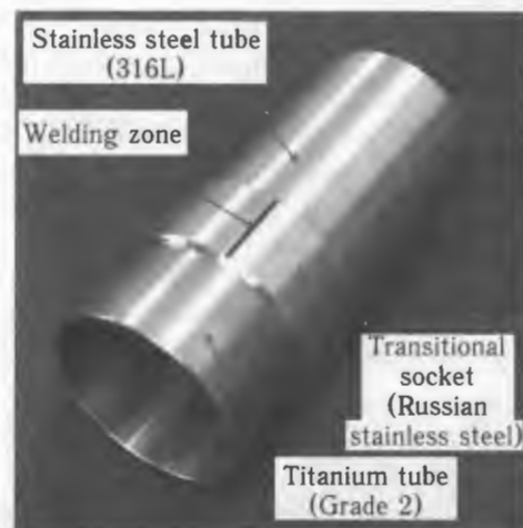
Stainless Steel + Titanium Bimetallic Tube installed into Cryomodule
