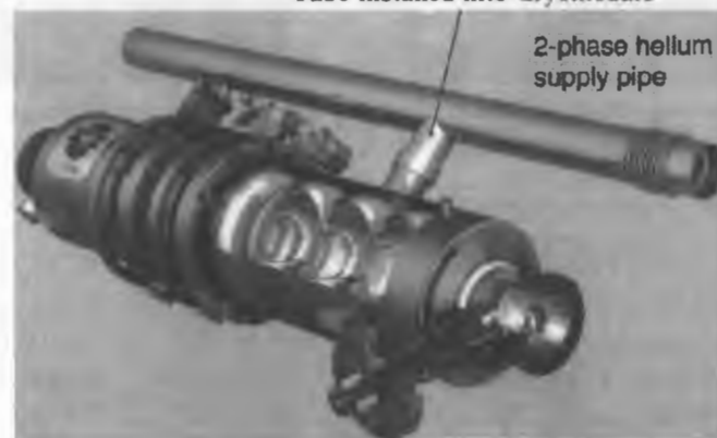
Stainless Steel + Titanium Bimetallic Tube installed into Cryomodule
