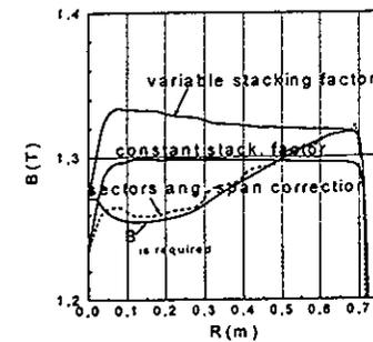
Figure 9: Radial dependence of the average magnetic field
