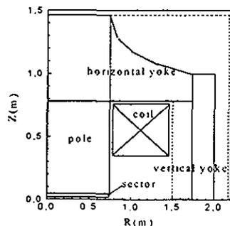
Figure 1: The view of the R-φ model for the cyclotron IC-35 magnet
