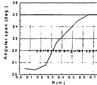
Figure 10: Radial variation of the sector angular span
