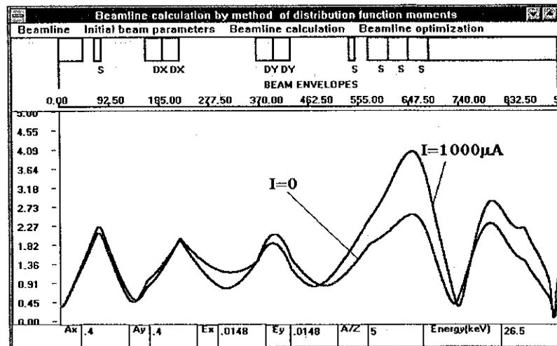
Figure 4: Vertical beam envelopes for  $A/Z=5$ ,  $I=0$  and  $I=1000 \mu A$ . No optimization has been made in solenoid strengths.
