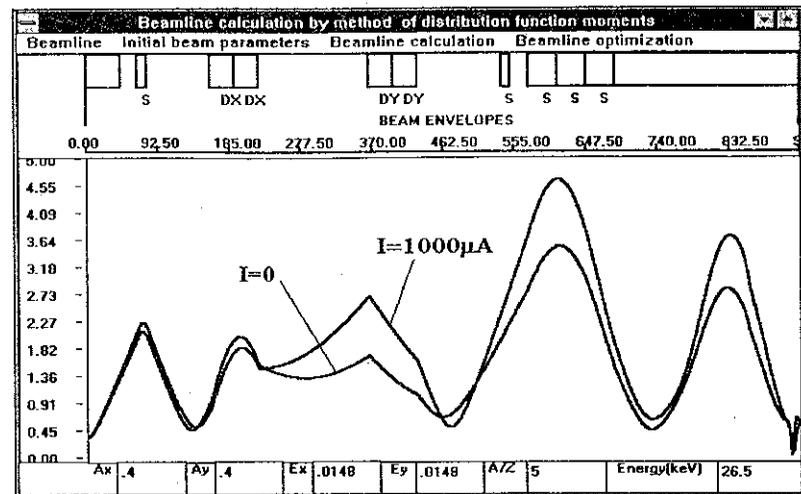
Figure 3: Horizontal beam envelopes for  $A/Z=5$ ,  $I=0$  and  $I=1000 \mu A$ . No optimization has been made in solenoid strengths.
