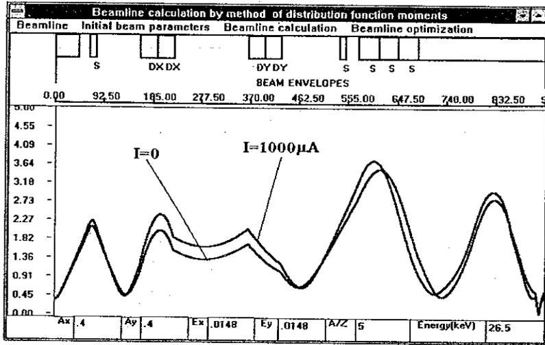
Figure 5: Horizontal beam envelopes for  $A/Z=5$  in the absence of space charge effects (curve marked by  $I=0$ ), and for current  $I=1000 \mu\text{A}$ . For the second case injection line has been optimized.
