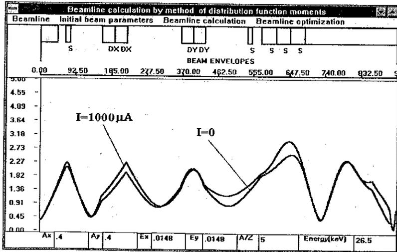
Figure 6: Vertical beam envelopes for  $A/Z=5$  in the absence of space charge effects (curve marked by  $I=0$ ), and for current  $I=1000 \mu\text{A}$ . For the second case injection line has been optimized.
