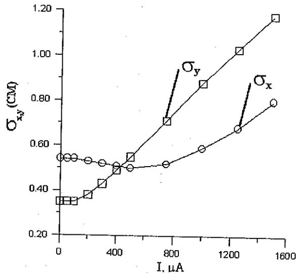
Figure 1: Dependences of the beam sizes at the end of injection line versus current for  $A/Z=5$ .
