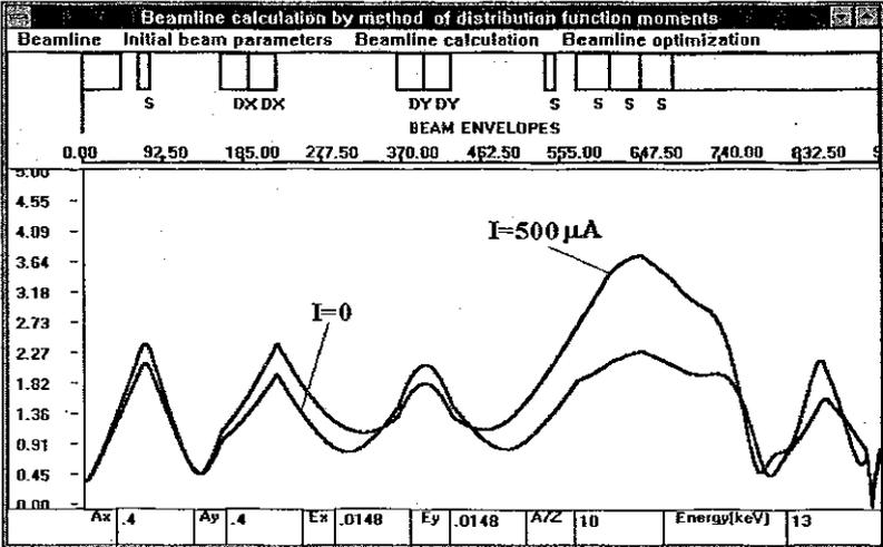
Figure 10: Vertical beam envelopes for  $A/Z=10$  in the absence of space charge effects (curve marked by  $I=0$ ), and for current  $I=500 \mu\text{A}$ . For the second case injection line has been optimized.
