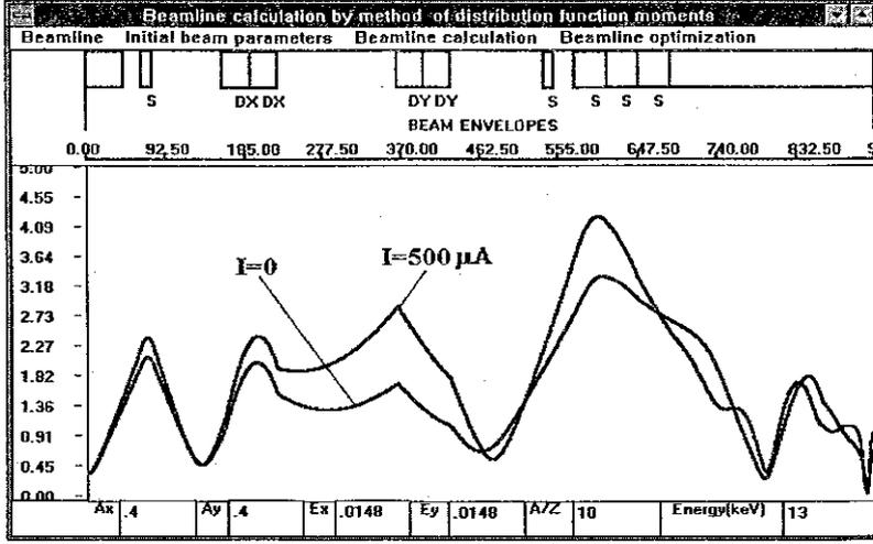
Figure 9: Horizontal beam envelopes for  $A/Z=10$  in the absence of space charge effects (curve marked by  $I=0$ ), and for current  $I=500 \mu\text{A}$ . For the second case injection line has been optimized.
