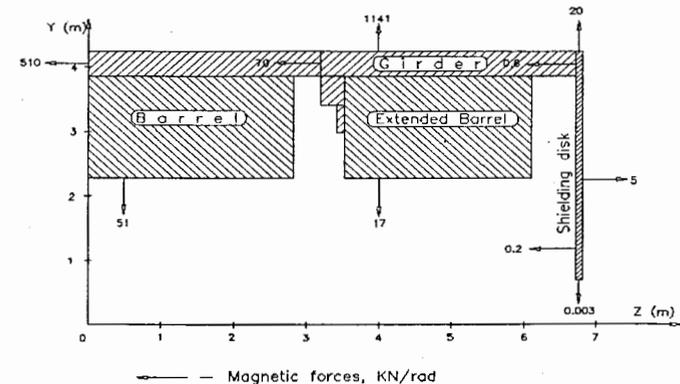
Figure 1 TileCal magnetic force distribution
