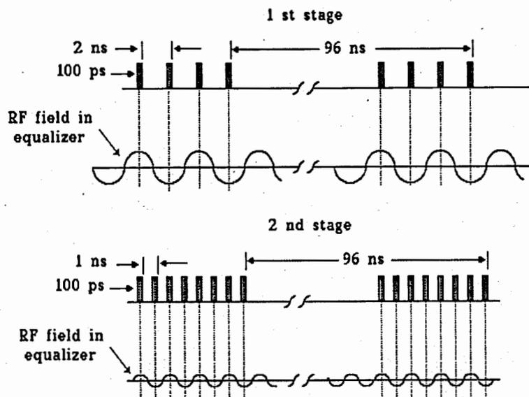
Fig. 8. The scheme of operation of the energy equalizers.
