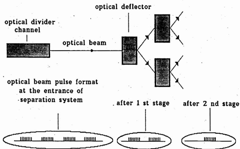
Fig. 13. The scheme of the optical beam separation system.
