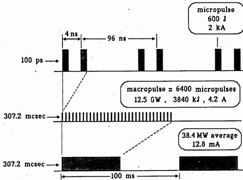
Fig. 6. Electron beam pulse format in RF accelerator.
