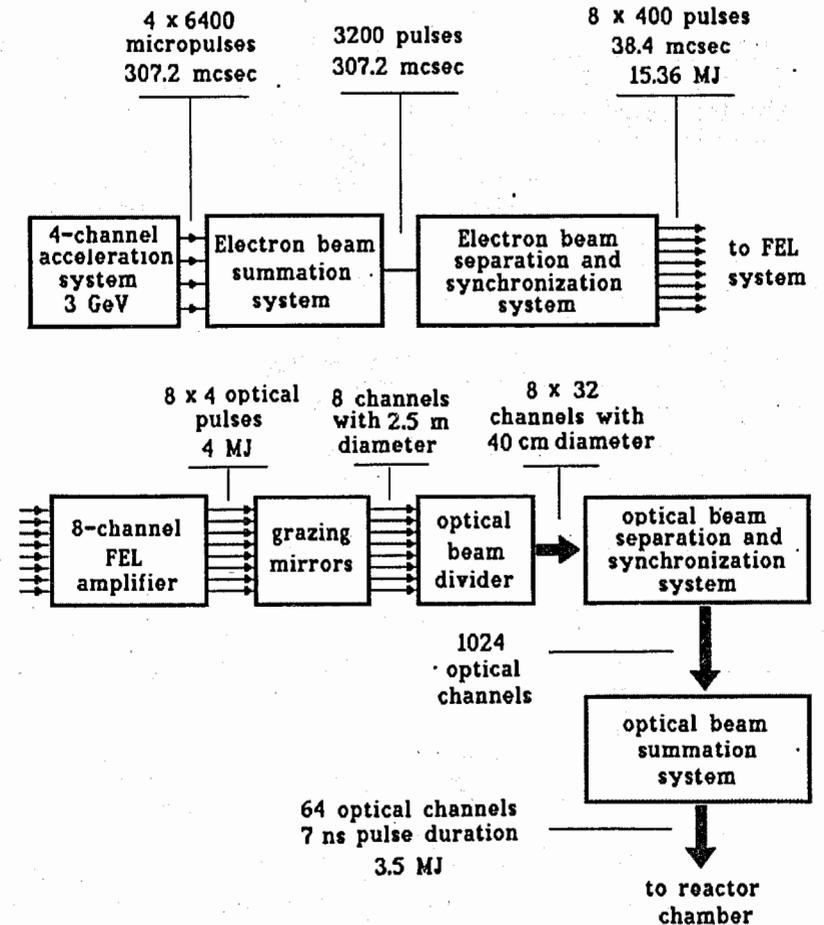
Fig. 3. The scheme of the FEL based energy driver.
