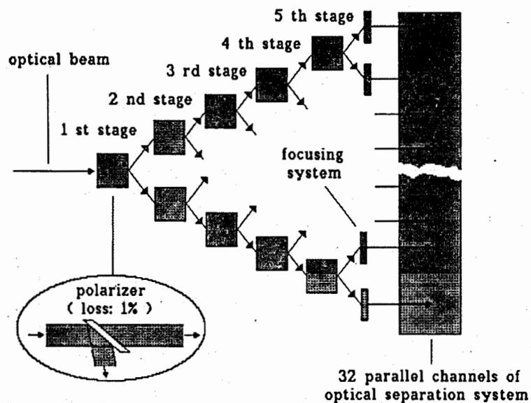
Fig. 12. The scheme of the optical beam divider.
