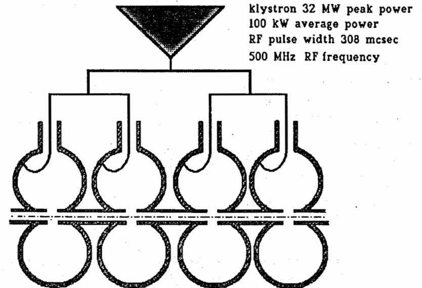
Fig. 5. Module of RF linear accelerator.
