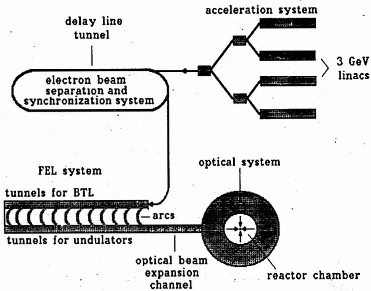
Fig. 4. Layout of the ICF reactor.
