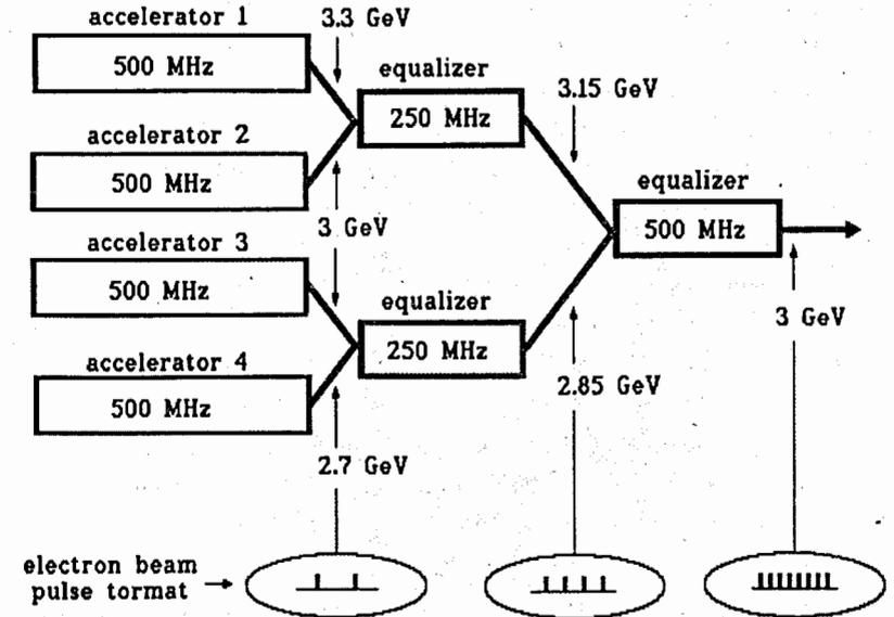
Fig. 7. The scheme of the electron beam summation system.
