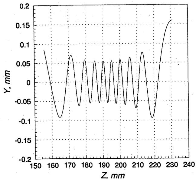
Fig.10. The trajectory of a 10 keV electron with an impact parameter of  $160 \mu\text{m}$  colliding with a proton bunch, Z-Y view. The proton bunch is moving to the right, and the electron is moving to the left. Plus/minus  $3\sigma$  of the proton bunch charge distribution in Z-direction is treated by the tracing code.
