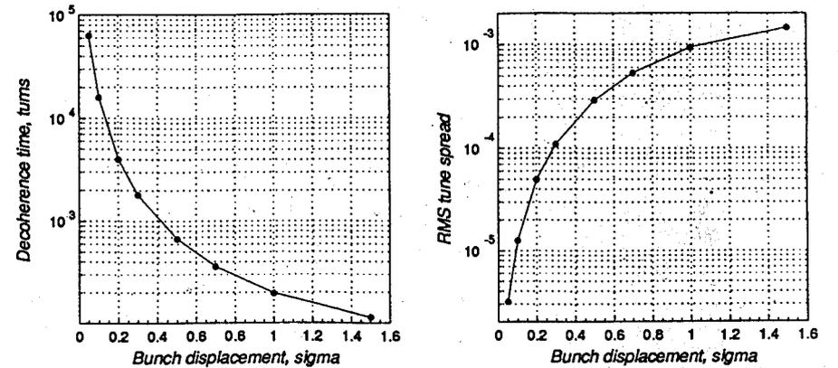
Fig.8. Decoherence time expressed in number of turns (left) and RMS tune spread of the beam particles (right) versus the electron beam displacement. The rightmost point corresponds to the case without compensation. The curve is drawn to guide the eye.
