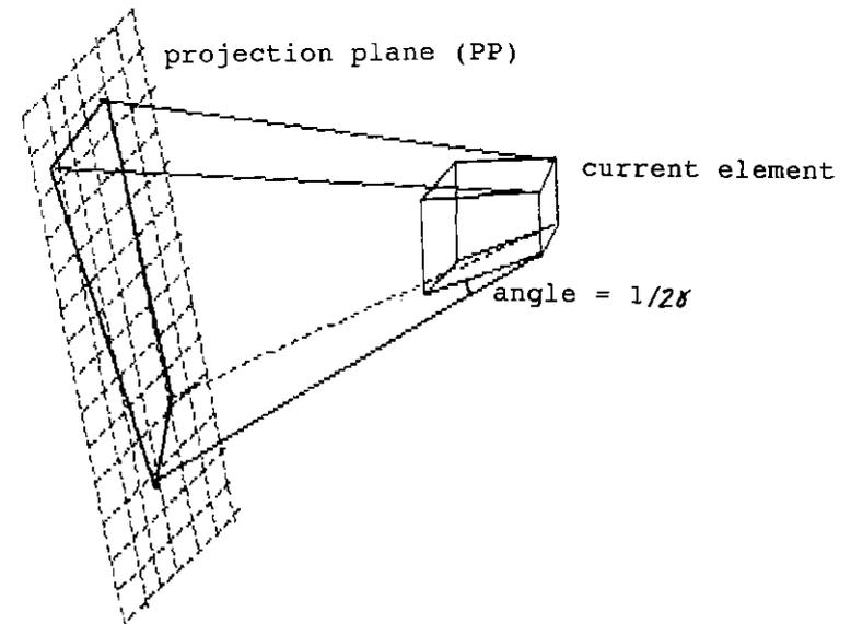
Fig.2 Mapping from a beam element  $dx dy ds$  to the PP with taking into account the vertical  $1/\gamma$  angle spread of the SR.
