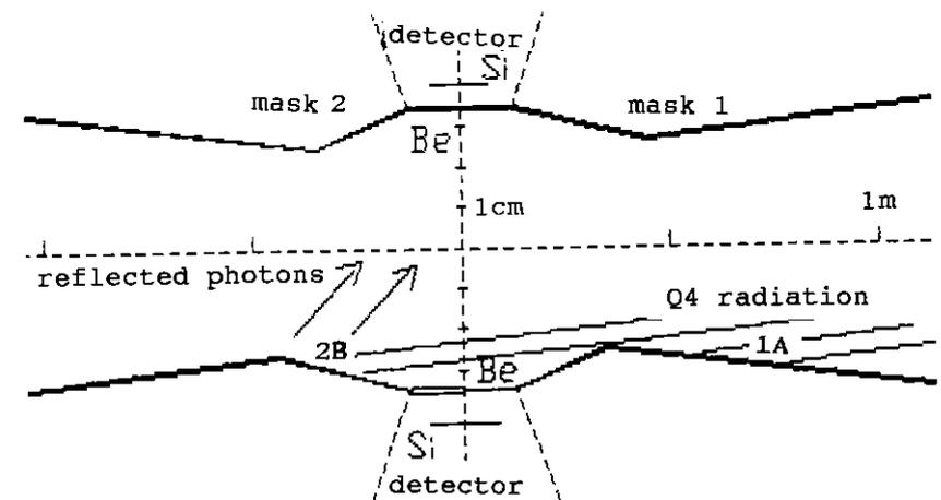
Fig.6 Variant 2 of masking (long asymmetric masks). The angle between the 2B side of mask 2 and the Y-axis is  $88.5^\circ$ . Photons reflected from side 1A ( $1.4 \cdot 10^{11}$  phot./s) and from the side 2B ( $6 \cdot 10^{11}$  phot./s) are incident on the Be surface. Of them  $5.2 \cdot 10^5$  phot./s enter the detector.
