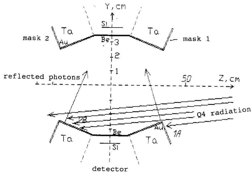
Fig.5 Variant 1 of masking (short symmetric masks). The angle between the 2B side of mask 2 and the Y-axis is  $87.5^\circ$ . Number of photons scattered from the mask-1 tip  $= 2 \cdot 10^7$ . Of them  $\sim 20$  phot./s enter the detector. Main background source ( $10^6$  phot./s) are the photons reflected from the side B2 ( $1.4 \cdot 10^{12}$  phot./s).
