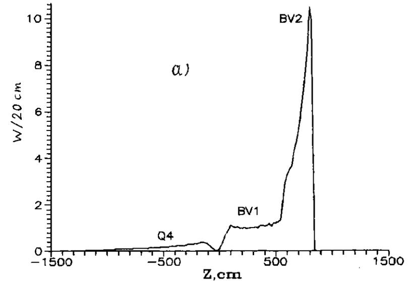
Fig. 3a Power density, deposited by one beam into the vacuum chamber wall (radius 6 cm):
