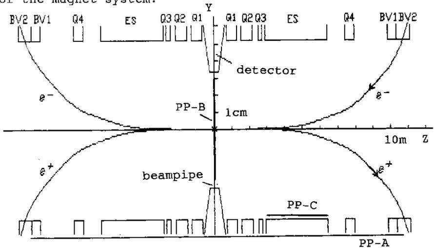
Fig.1 Layout of the magnetic elements in the interaction region (IR) of the Tau-Charm factory. Several positions of the SYNRAD projection plane are shown: PP-A, PP-B, PP-C.
