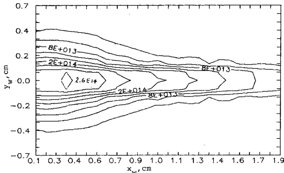
Fig.4 SR intensity incident on the PP-B in units number phot. > 1 keV/s/mm<sup>2</sup>, produced by the set of low  $\beta$  quadrupoles Q1, Q2, Q3.
