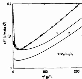
Fig. 4. The specific heat capacity plotted as  $c/T$  vs  $T^2$  for  $\text{YBa}_2\text{Cu}_3\text{O}_7$ . Points: this work, 1 - Phillips et al.<sup>1)</sup>, 2 - Junod et al.<sup>2)</sup>
