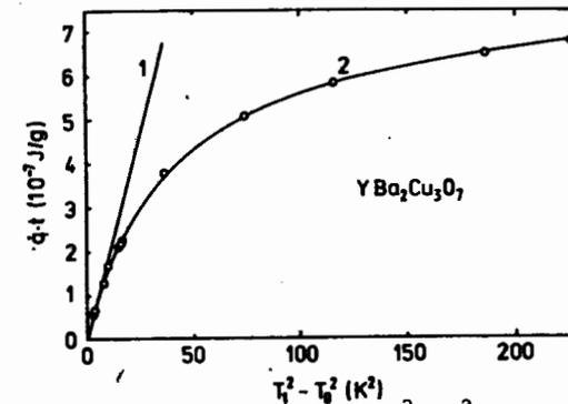
Fig. 3. The value  $\dot{q} \cdot t$  as a function of  $T_1^2 - T_0^2$  ( $T_0 = 1.5$  K),
