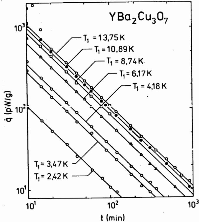
Fig. 2. The specific power released in  $\text{YBa}_2\text{Cu}_3\text{O}_7$  after cooling from various  $T_1$  to  $T_0 = 1.5$  K as a function of time. Straight lines:  $\dot{q} \sim t^{-1}$
