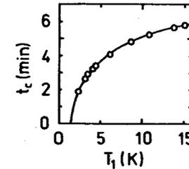
Fig. 1. The time  $t_c$  required for cooling the specimen from  $T_1$  down to  $T_0 = 1.5$  K
