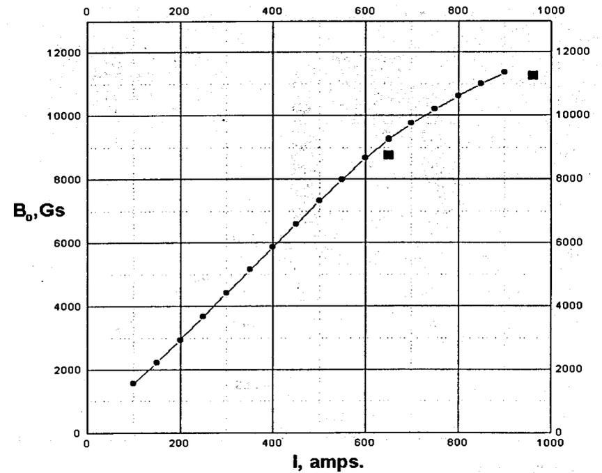
Fig.5. The magnetization curve of the magnet M2: the squares represent theoretical calculations, circles – experimental data.
