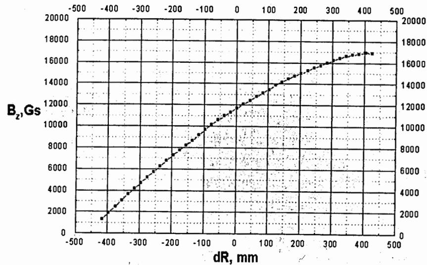
Fig.7. The magnetic field distribution in the central section of the magnet M2 for the field level  $B_0=11600$  Gauss. The measured points coincide with the values, calculated according to the equations (3) and (4) [3], with the accuracy better than 2.0%.
