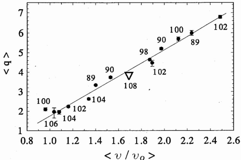
**Fig. 1.** The velocity dependence of the average charge states  $\langle q \rangle$  of very heavy atoms traversing 1 Torr of hydrogen. Z values for atoms are given near the data points. The systematics is based on both previous data [1,18] and  $\langle q \rangle$  measurements performed in this work. The triangle shows the  $\langle q \rangle$  value for Z=108. The line is included to guide the eye.
