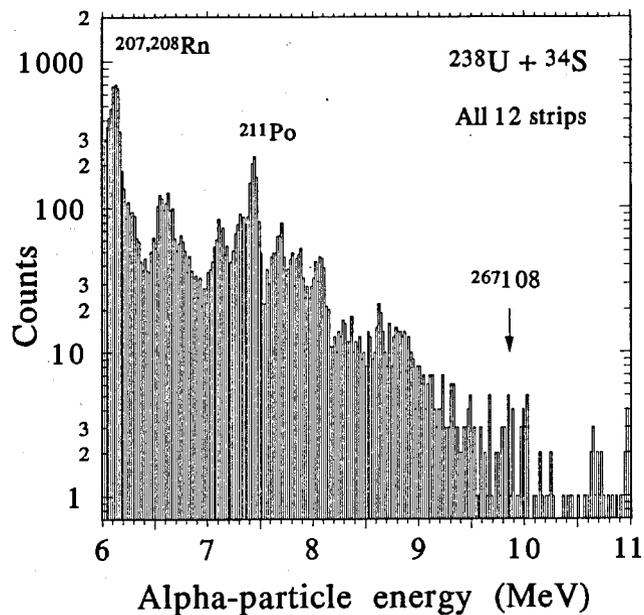
**Fig. 2.** Energy spectrum of out-of-beam  $\alpha$  particles detected in all 12 strips in the 36-day bombardment of  $^{238}\text{U}$  with  $1.7 \times 10^{19}$  particles of  $^{34}\text{S}$ . Most  $\alpha$ -activities seen in the spectrum are due to  $Z \geq 84$  nuclides produced in deep inelastic collisions between  $^{238}\text{U}$  and  $^{34}\text{S}$ , with possible traces of some  $\alpha$  emitters from  $^{nat}\text{W} + ^{34}\text{S}$  calibrations.
