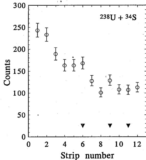
**Fig. 3.** The distribution across detector strips for all out-of-beam  $\alpha$ -decay events with  $E_{\alpha} = 7.6$  to  $10.4$  MeV detected in the  $^{238}\text{U} + ^{34}\text{S}$  bombardment. The triangles show the location of the three  $Z=108$  event sequences.
