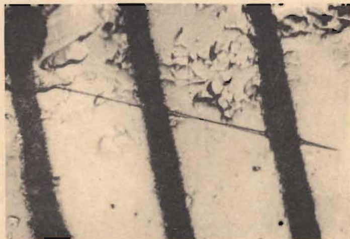
Fig. 2. a) Photograph of the annealed olivine crystal bombarded with a laser beam. b) Photograph of the annealed olivine crystal bombarded with ^{60}\text{Ni} ions through a system of slits.
