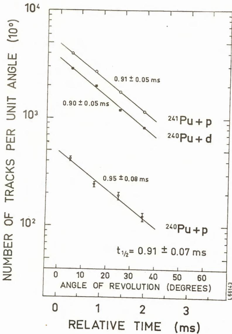
Fig.2 Decay curves for <sup>240m</sup>Am produced by three different reactions. The conversion from angle of revolution to time is based on measurement of the rotation frequency of the wheel.
