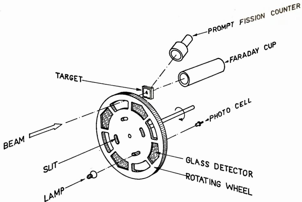
Fig.1 Schematic diagram of the irradiation chamber. The target is stationary. The rotating wheel serves three purposes (I) it brings the glass detectors recording delayed fission fragments in front of the target in the intervals between the beam bursts, (II) by the aid of the slits and the photocell, it provides a pulse which is used to switch the beam off just before the glass plate moves in front of the target, and (III) it prevents any residual beam which
