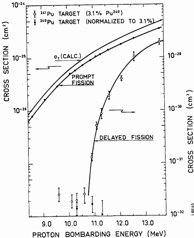
Fig.3 Excitation function for prompt and delayed fission resulting from proton bombardment of  $^{241}\text{Pu}$ , see text.
