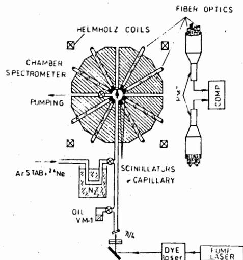
Fig. 3. Experimental lay-out for the measurement of the asymmetry of  $\beta$ -particle emission with respect to the nuclear spin.
