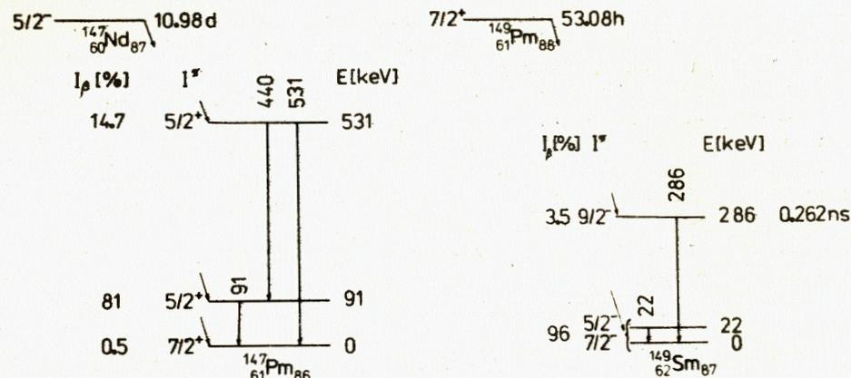
Fig.1. Parts of  $^{147}\text{Nd}$  and  $^{149}\text{Pm}$  decay schemes relevant to present work.
