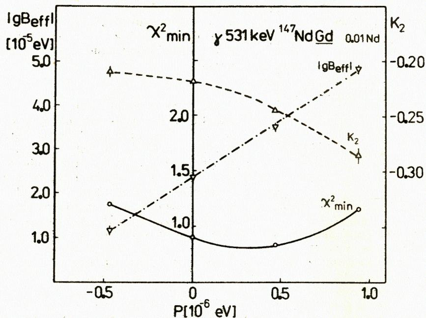
Fig.5. Results of the  $\chi^2$ -analysis of measured temperature dependence of fig.3. For obtaining of  $G_2$ -factor we could consider only values of  $|P| \leq 10^{-7}$  eV estimated on the basis of measured<sup>23/</sup> values of electric quadrupole hyperfine splitting constants for  $^{143,145}\text{NdGd}$  and ground state electric quadrupole moments of  $^{143,145,147}\text{Nd}$  quoted in<sup>24/</sup>.
