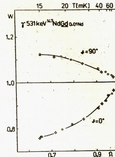
Fig. 3. Normalized intensity  $W(0^\circ, T)$  of 531.0 keV gamma-ray of  $^{147}\text{Nd}$  plotted versus normalized intensity  $\Omega(0^\circ, T)$  of 834.8 keV gamma-ray of  $^{54}\text{MnNi}$  nuclear orientation thermometer.
