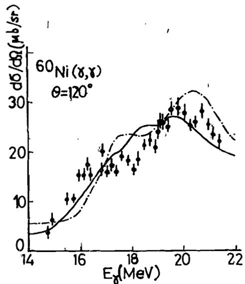
Fig. 2. Differential cross sections of elastic dipole photon scattering by the GDR in  $^{60}\text{Ni}$ . The points are the experimental data<sup>15,16</sup>. The solid and dash-dotted lines are the results of QPM calculations.
