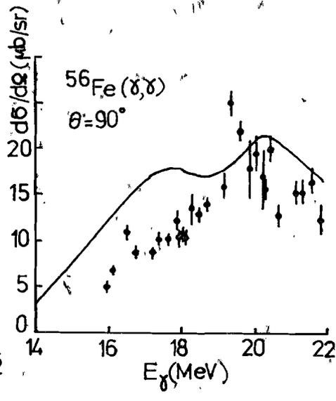
Fig. 3. Differential cross sections of elastic dipole photon scattering by the GDR in  $^{56}\text{Fe}$ . The points are the experimental data<sup>16</sup>. The solid line is the QPM calculation.
