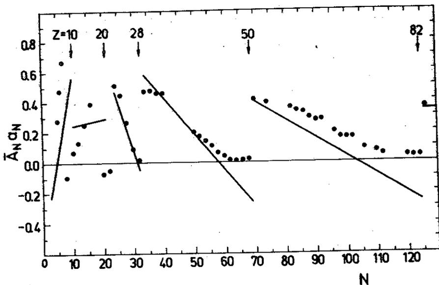
Fig.3. The  $\bar{A}_N a_N$  slopes of normalized RMS radii for isotonic sequences multiplied by the average mass numbers  $\bar{A}_N$  as a function of neutron numbers. The solid lines show the result of a weighted least-squares fit to  $\bar{A}_N a_N$  values derived from experimental data<sup>18/</sup>. Circles denote the calculated values.
