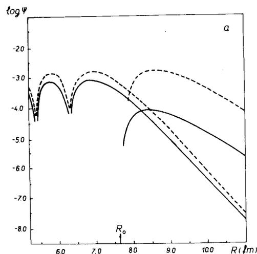
Fig. 3. The comparison of functions  $\psi_{RNL}^{SM}(R)$  and  $\psi_c(R)$  for  $\alpha$ -transitions of  $^{210}\text{Bi}$  nucleus:  $1^- \rightarrow 1^-$  ( $L=0$ )-dotted lines and  $9^- \rightarrow 2^-$  ( $L=8$ )-solid lines. The functions  $\psi_{RNL}^{SM}$  are labeled by number 1, the functions  $\psi_c$  - by number 2.
