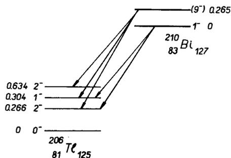
Fig. 1. Energy levels of  $^{206}\text{Tl}$  and the alpha decay scheme of  $^{210}\text{Bi}$ .
