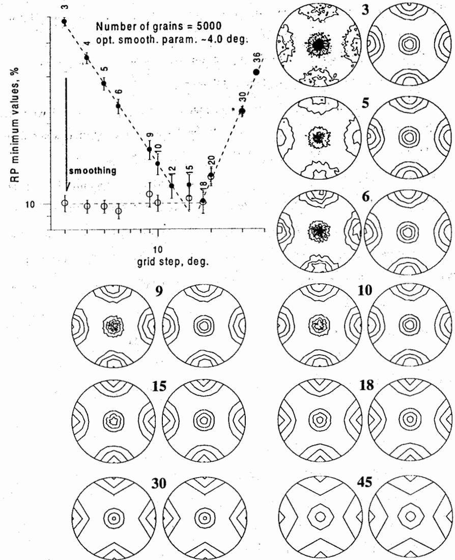
Fig.2. The dependencies of the RP-value before pole figures smoothing (dashed circles) and the minimum achieved RP-value after optimal smoothing (clear circles) on the grid parameter of the net used. As an illustration, the pairs unsmoothed-smoothed pole figures (100) are plotted.
