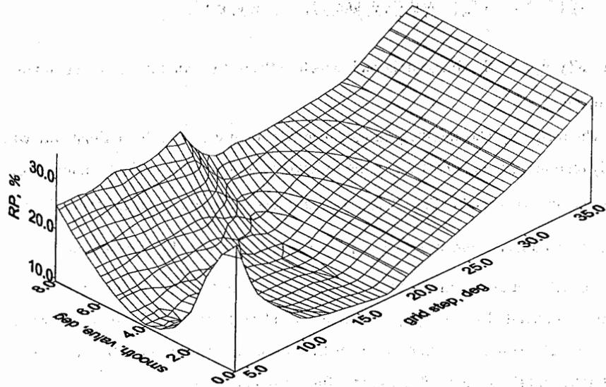
Fig.1. The dependence of the RP-value on the smoothing parameter and the grid parameter plotted as a surface (bottom) and as its sections (top).
